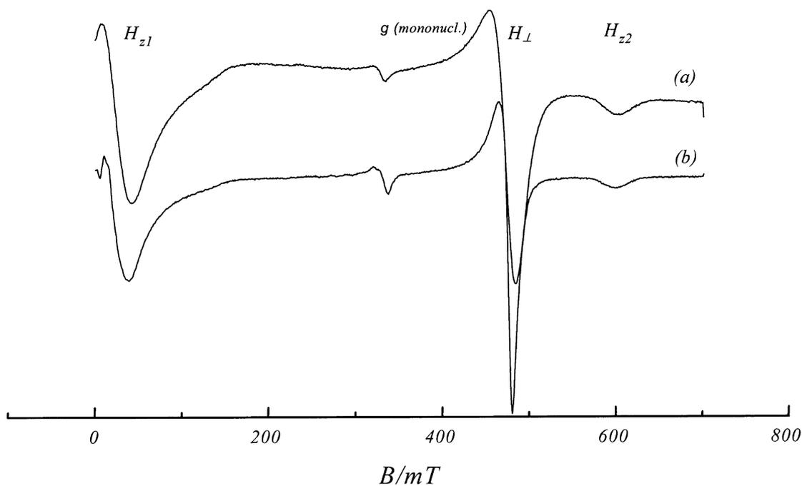
Fig. 4. EPR spectra of **1A**, recorded at (a) room temperature and at (b) 150 K.
