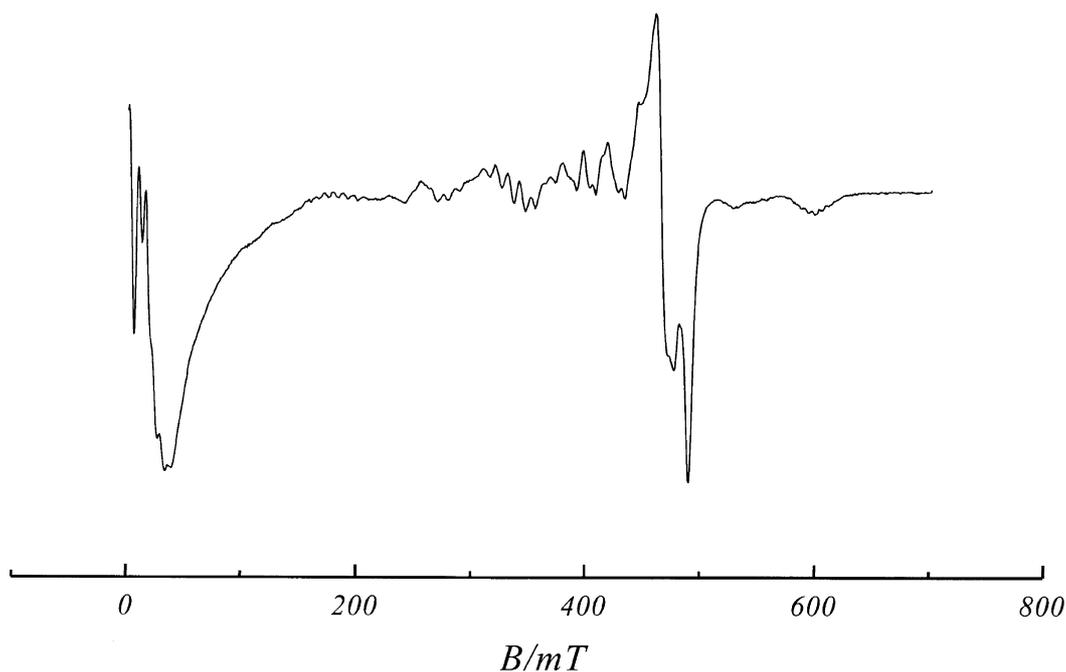
Fig. 5. EPR spectrum of **3**, recorded at 150 K.
