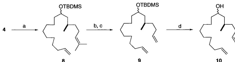
**Scheme 2.** Reagents and conditions: (a) TBDMSCl, imidazole, DMF, 21 h; (b) O<sub>3</sub>, CH<sub>2</sub>Cl<sub>2</sub>, -78°C, Me<sub>2</sub>S, -78°C then rt, 12 h; (c) Ph<sub>3</sub>PMeBr, *n*-BuLi, THF, -78° then rt, 4 h; (d) TBAF, THF, 24 h.
