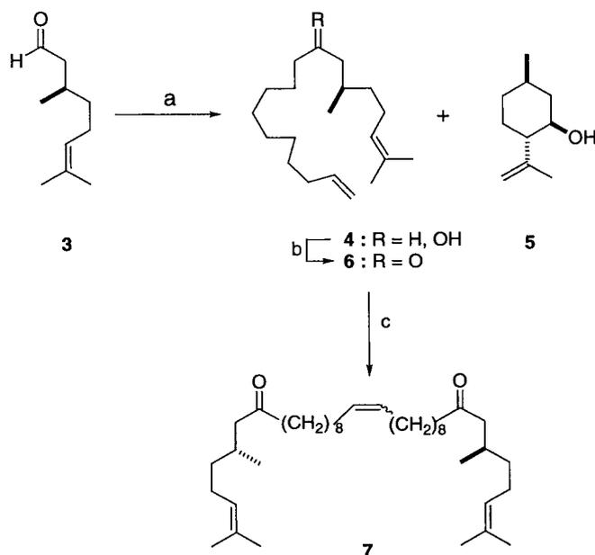
**Scheme 1.** Reagents and conditions: (a) 10-bromodec-1-ene, Mg, Et<sub>2</sub>O, 16 h; (b) Jones reagent, CH<sub>3</sub>COCH<sub>3</sub>, 10 min; (c) 5 mol% of **2**, 21 h, 45°C.
