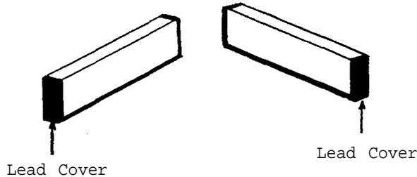
Nail thin strips of lead along the sides and base of the pieces of wood (D, E, F and G) to prevent them from floating in the ripple tank. The weighted pieces serve as suitable barriers.
