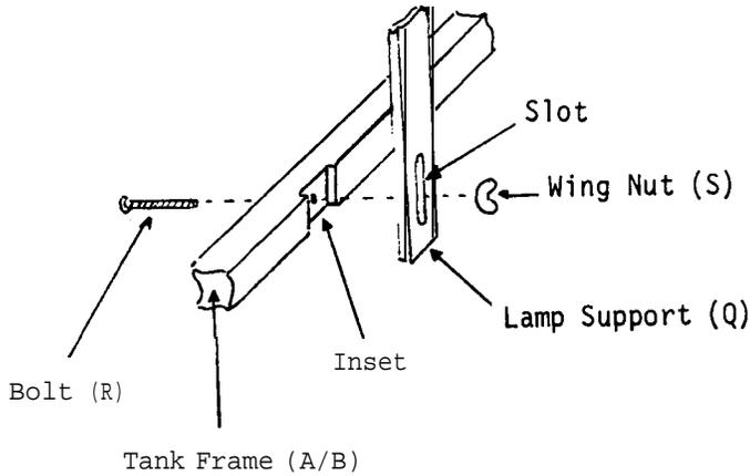
The vertical component of the lamp support is made, and attached to the ripple tank, in very much the same way as the legs. Drill and chisel a slot (7 cm x 0.5 cm) near to the bottom of end wood (Q) to permit adjustment. Attach the support to the ripple tank frame with bolt (R) passed through the lower part of the frame, and held in position by wing nut (S).
