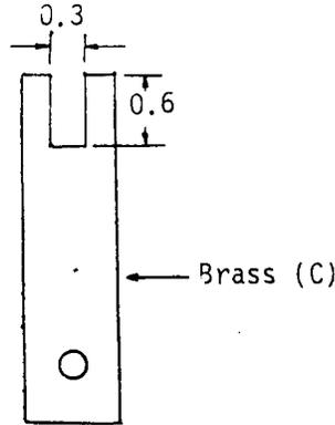
Cut four clip holders from the four brass sheets (C), making a screw hole at one end and a small slit at the other. Fit the four slits in the holders under the locking nuts of the four terminals of the multipurpose coils (B). Then position each coil in turn on the upright so that the pole head is at exactly the same height above the base as the moving coil core. In this position screw the clips firmly onto the edge of the upright with the screws (D).
