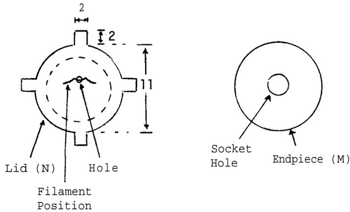
to filament. Ideally the filament should be a straight line, but a slightly bent filament such as that illustrated will serve the same purpose.
