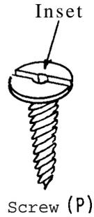
Insert the wood screw (P) into the base at a point 2 cm from the front of the upright and centered. Drill an inset (0.2 cm deep) into the head of the screw so that it will serve as a lower pivot for the coil.
