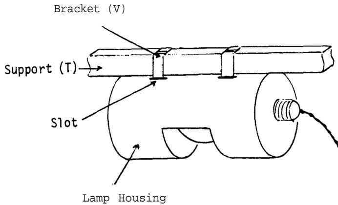
pass the steel strips through. Fasten the loose ends of the brackets together with folded pieces of aluminum (W). Then slide the brackets over the lamp support.
