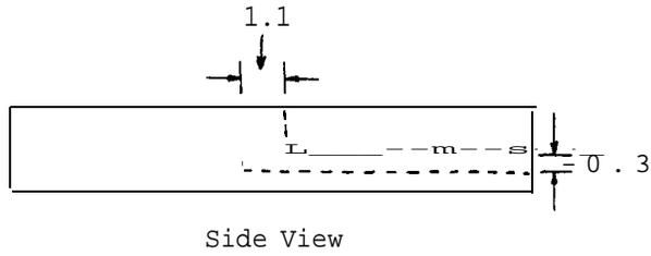
Drill a vertical hole (1.0 cm diameter, 1 cm deep) into the middle of the top surface of the wood (P). Drill a horizontal hole (0.3 cm diameter) into the middle of one end of the block, so as to meet the first hole.
