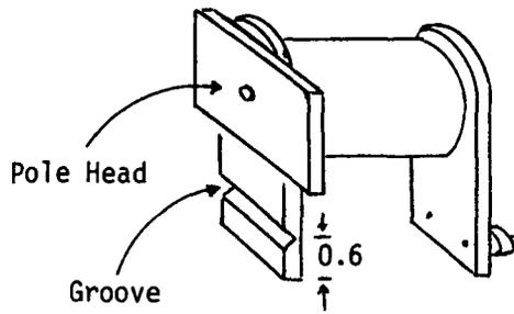
Make two Multipurpose Coils (B), complete with pole heads, as described under IX/A2. Cut a horizontal groove in the front endpiece of each (just beneath the pole heads) to insure a good grip for the coil holders.
