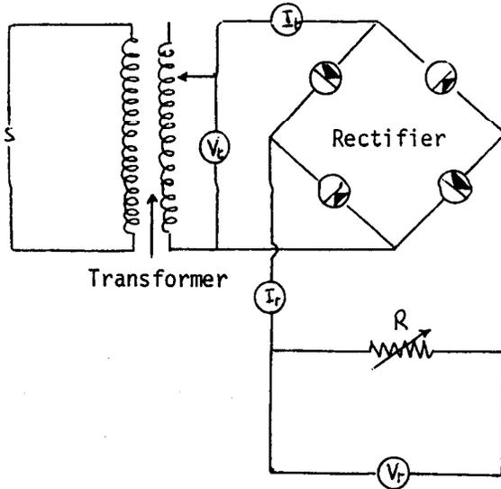
noted that the output voltage ( $V_r$ ) fell off as the resistance decreased. [A very small proportion of the fall in voltage may be attributed to the drop in voltage ( $V_t$ ) from the transformer.]
