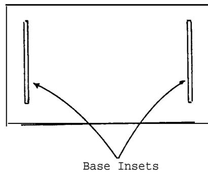
Make two insets (8 cm long, 0.5 cm wide, 0.2 cm deep) in appropriate positions on the base to hold the endpieces. Fix the endpieces firmly in the insets with wood cement.
