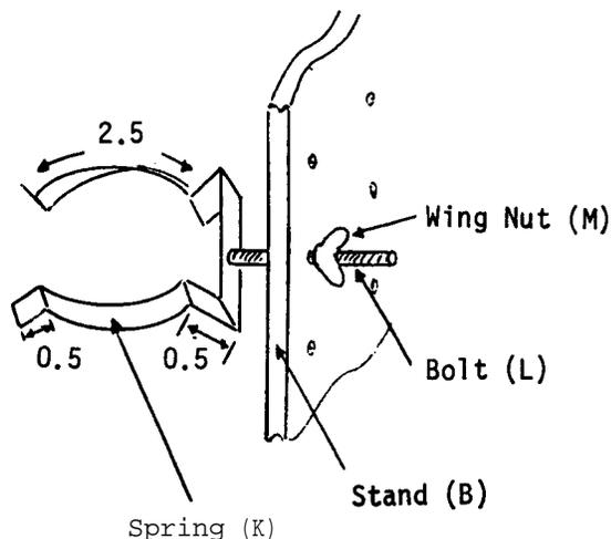
Take a length of packing case steel band (K) and drill a hole (diameter 0.3 cm) through its center. Then bend it as indicated into the form of a spring clip. This size of spring clip is suitable for a standard test tube. Attach this to the support stand with a bolt (L) and wing nut (M). Two identical spring clips should be made.
