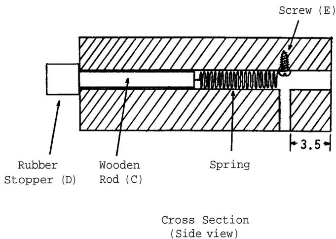
Bore a hole into the bottom of the cart body so that it meets the bore hole for the spring 3.5 cm from the end of the body. Then insert the screw (E) to anchor the loop end of the spring.
