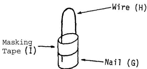
Cut two lengths from the nail (G), one 1.0 cm long and one 2.0 cm long. Attach a three centimeter-long loop of the magnet wire to the end of each nail with the help of a strip of masking tape
