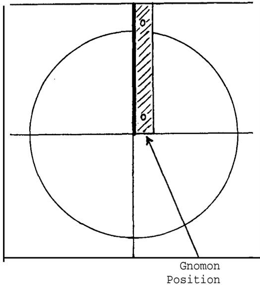
Cut the base from the wood (A). Use a felt pen to mark off the surface of the base into four equal portions. Draw a circle (diameter 7 cm) on the base with its center at the middle of the base.
