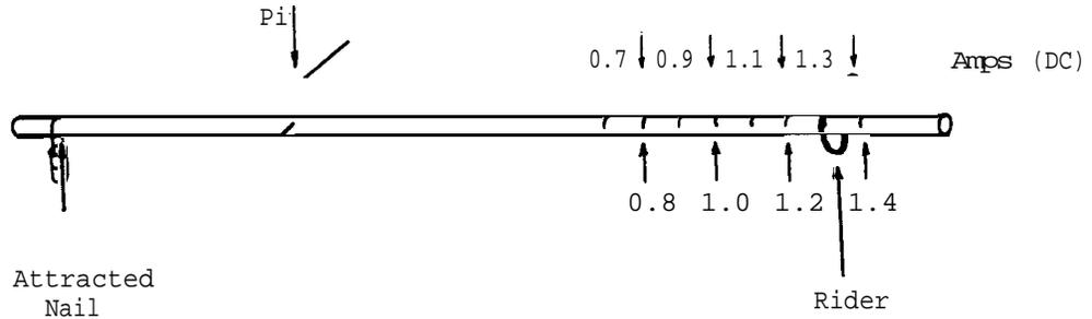
(iii) The resultant scale on the straw is linear. **In other** words, doubling the current passing through the coil doubles the force exerted by the coil on the nail, and the distance between the rider and pivot must be doubled to reestablish the balance of the straw.
