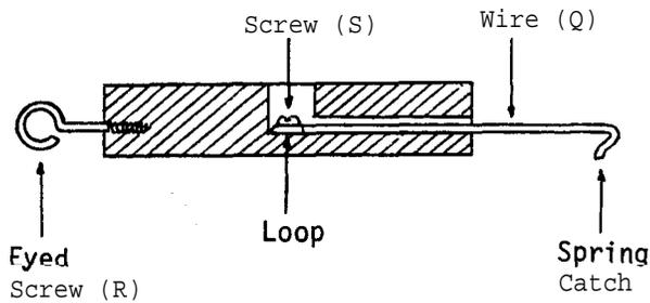
Clean the surface of the wire (Q) with sandpaper. Insert one end of the wire fully into the horizontal hole, and using a pair of dog-nosed pliers (inserted through the vertical hole) bend a loop into the inserted end of the wire. Insert a small screw (S) through the loop to attach the wire **permanently** within the block.
