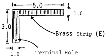
Take the two brass strips (D) and drill a hole (0.3 cm diameter) close to the end of each. Insert the strips under the supports (C) at one end of the base as indicated. Use bolts (F) and nuts (G) to make four terminals (F/G) as described under VIII/A2 Component (4). Fit two of the terminals on the base so that each is connected to a brass strip by means of the appropriate hole.
