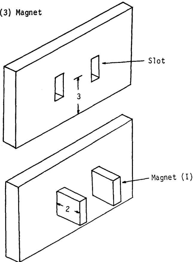
Obtain a strong horseshoe magnet (I) in which the separation of the two sides of the horseshoe is approximately 3 cm (or a little more). Make slots in the upright (B) as illustrated to allow the magnet to be pushed through the upright so as to protrude a distance of 2 cm. Once the moving coil (below) has been fixed finally in position, fix the magnet firmly in the upright with epoxy resin. The slots are most easily made before the upright has been screwed to the base.
