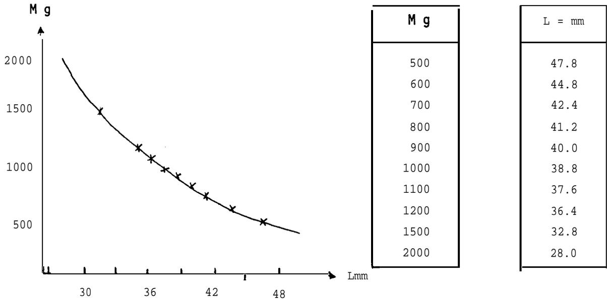
(iii) Because of friction between the plunger and the sides of the column, the syringe tends to be insensitive to weights of less than about 500 g, but it readily measures weights from this lower limit up to around 5,000 g.
