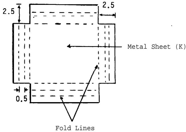
Cut the corners (2.5 cm x 2.5 cm) out of the aluminum sheet (K), and fold the projections as illustrated so that they may be bent over the wire frame to form a suitable scale pan.
