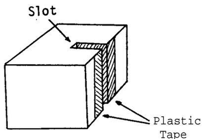
Alternatively, cut a slot (0.2 cm wide) in a wooden block (2 cm x 2 cm x 2 cm). Line the slot with plastic tape to prevent the wood from scratching the surface of the mirror to be held.
