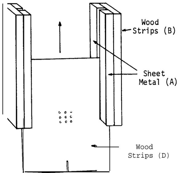
Nail or glue two wood strips (B) to a third strip (C), leaving about a 0.1 cm gap between them. Make an identical piece from the other two narrow strips (B) and the one remaining wide strip (C). Slide the metal sheet into position between the two pieces.
