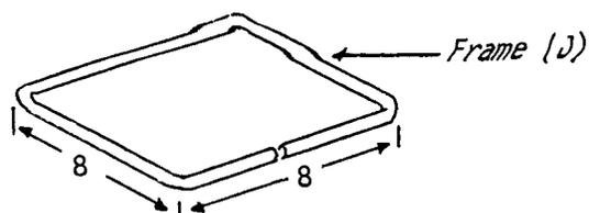
Make a frame for the scale pan out of aluminum or galvanized wire (J).
