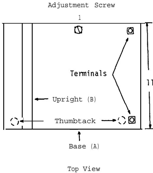
Make two terminals in the front of the base from the brass bolts (D) and nuts (E) [See VIII/A2, Component (4)].
