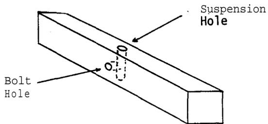
In each wood holder (G), drill a vertical suspension hole (0.2 cm diameter) and a horizontal bolt hole (0.3 cm diameter) to meet the vertical hole.
