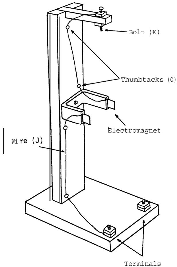
Drill two holes (0.3 cm diameter) into the front of the base. Make two terminals from the nuts (N) and bolts (M) as described under item VIII/A2, component (4). Set the terminals into the holes, making sure they are inset into the bottom of the base, thus leaving the bottom perfectly smooth.
