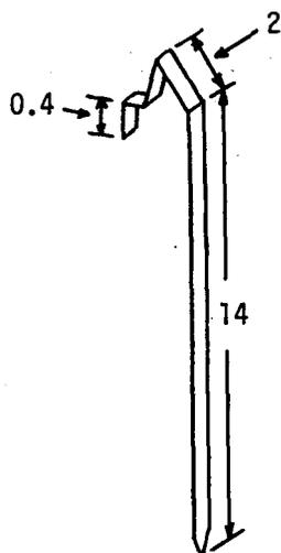
Take a sheet of aluminum (E) and bend it into the shape of a pointer as illustrated. Then attach the pointer to the arm just above the pivot.
