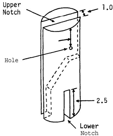
Make a support from a wooden dowel (E) as indicated. Cut a lower notch in the support to enable it to sit on the side of the upper reservoir (A). Make an upper notch to permit the full movement of the pointer (E) to be attached. Drill a hole (0.2 cm diameter) horizontally through the upper part of the support to permit passage of the nail (G) to serve as the pivot for the lever.
