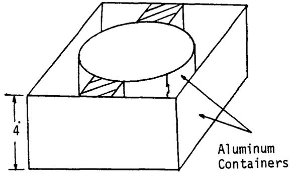
container. Cover the nail ends at both extremities of the containers and the wooden rods. You will now have two pole heads.
