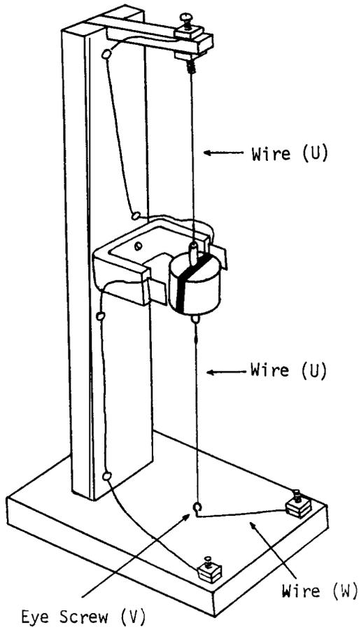
Bare one of the ends of the magnet wire (U) and wrap it around the eye of the needle in the top end of the dowel (S). Suspend the dowel and coil by the wire, so that the dowel hangs between the pole ends of the electromagnet. With the dowel in this position, fasten the other end of the magnet wire to the hole in the bolt in the wire support (after cleaning the end of the magnet wire).
