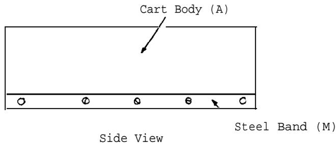
Drill two horizontal holes (0.5 cm in diameter) through the cart body to permit passage of the front and rear axles. Make these holes 1.0 cm from each edge of the cart body (A). Cut the chassis from metal packing case bands (M). Drill five holes along the length of the
