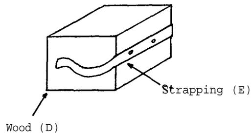
Bend a length of packing case steel (E) as shown and nail it to the side of the wooden block (D).
