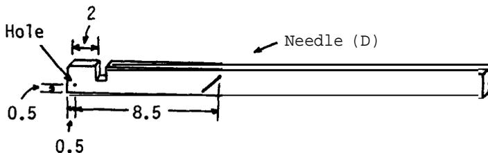
Make the balance arm from the soft wood (C). Drive the needle (D) horizontally through the arm 9 cm from one end and 0.5 cm from the top surface. Cut a notch (0.5 cm wide, 1.0 cm deep) in the top of the arm and drill a small hole (0.2 cm diameter) through the corner of the wood.
