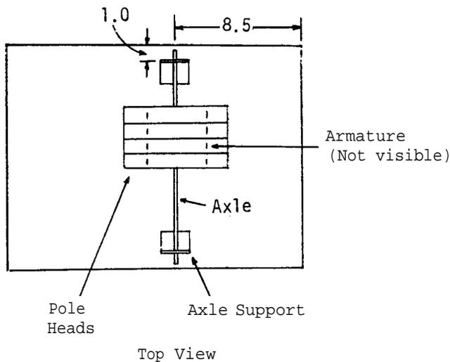
Slide the supports on to either side of the axle (B), and attach them firmly to the base of the apparatus in the position shown.
