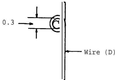
Make two vertical supports for the coil by twisting the coat hanger wire (D) into the shape indicated. Set the supports vertically upright in the newly drilled holes in the base.
