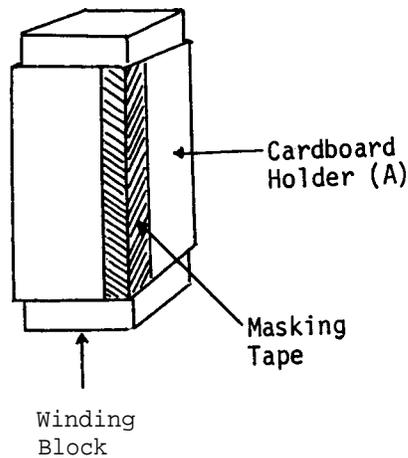
Wrap the cardboard around the block, fastening the two loose edges together with masking tape (D), thus producing a cardboard holder on which to wind the coils.
