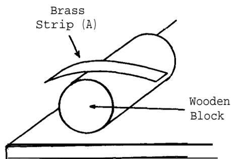
Cut the sheet of brass (A) on a metal guillotine (to be found in your nearest metalwork shop). If the metal sheet is cut with bench sheers some distortion is almost certain to result, thus lowering the quality of the mirror. If the mirror is to be curved, bend it over a smooth, curved, wooden block until the mirror becomes the arc of a circle of radius 8.5 cm.
