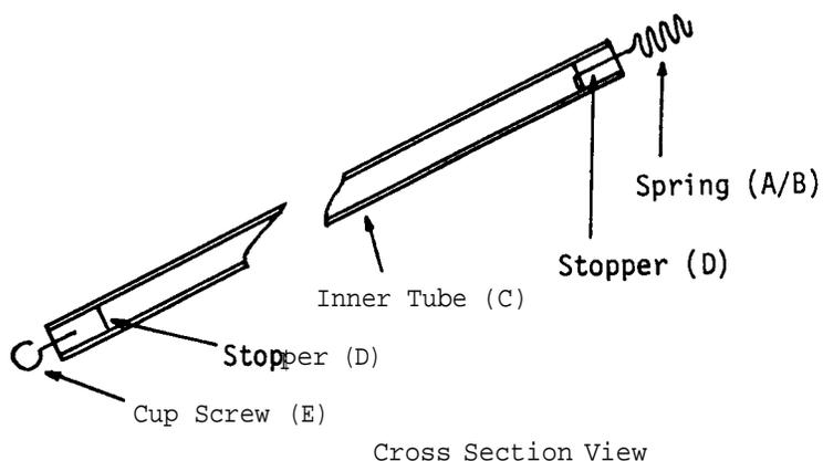
Make two stoppers out of the wood (D). Fix a cup screw (E) into one of the stoppers and glue it permanently into one end of the aluminum tube (C). Drill a small central hole through the other stopper (D) and insert the straight end of the spring, bending the end over to hold it in position. Glue the stopper into the other end of the tube.
