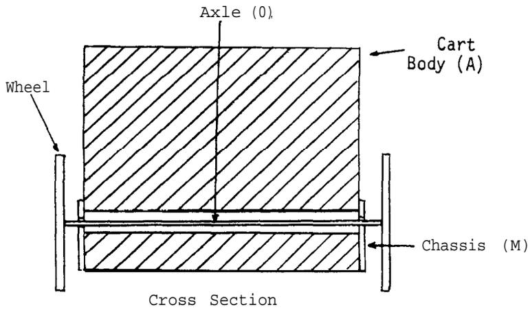
strip, two (diameter 0.3 cm) to coincide with the centers of the axle holes and three to enable the strip to be attached firmly to the body with screws.
