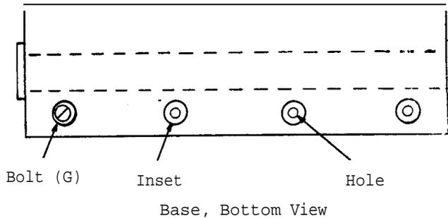
Make four insets (0.2 cm deep) at equal intervals underneath the front side of the base to take the boltheads of the terminals. Insert the four bolts (G) from below, through holes drilled through the base, and attach the locking nuts (H) and terminal nuts (H).
