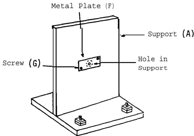
Drill a hole (diameter 0.5 cm) through the exact middle of the vertical component (A) of the support. Drill a hole (diameter 0.2 cm) through the center of each of the aluminum plates (F) to serve as pivot holes for the pointer. Drill two holes (diameter 0.2 cm) in diagonally opposite corners of each plate, so that the latter may be screwed onto either side of the support over the centrally drilled hole. The holes in the plates should be at the same height on both sides of
