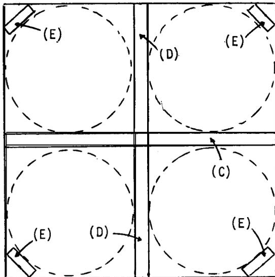
Nail wood strips (C,D) to the top of the plywood sheet (B) so as to divide it into four equal portions. Nail the wood strips (E) at the corners of the plywood in such a way that the four cell containers, placed in the appropriate quarters, will be held in position on the plywood base.
