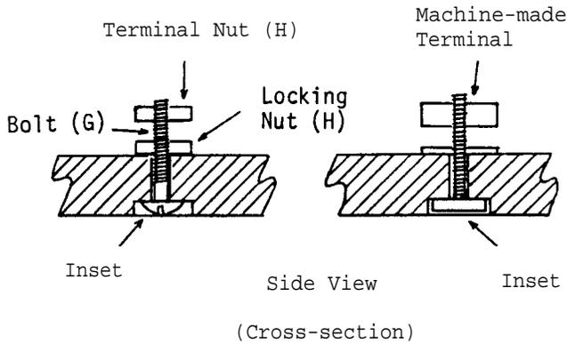
Make four terminals from the brass bolts (G) and nuts (H). Two nuts are required for each terminal, one to serve as a locking nut and one as a terminal nut.
