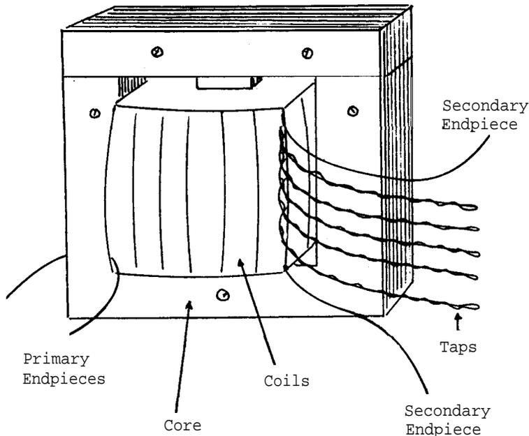
Assemble the coils on the W-shaped core, using paper or wood wedges if necessary to insure the coil is held firmly on the central upright of the core.
