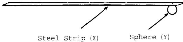
The steel strips (X), or stiff coat hanger wire, will serve as the arms of the vibrator. Attach a glass sphere (Y) to the end of each arm using epoxy resin.
