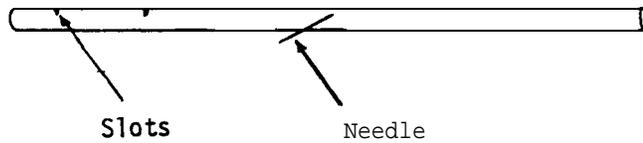
to the top surface of the straw, thus lending stability to the balance arm. Use a razor blade to cut small V-shaped slots in the top surface of the straw at regular intervals of 2 cm. Balance the straw on top of the support.
