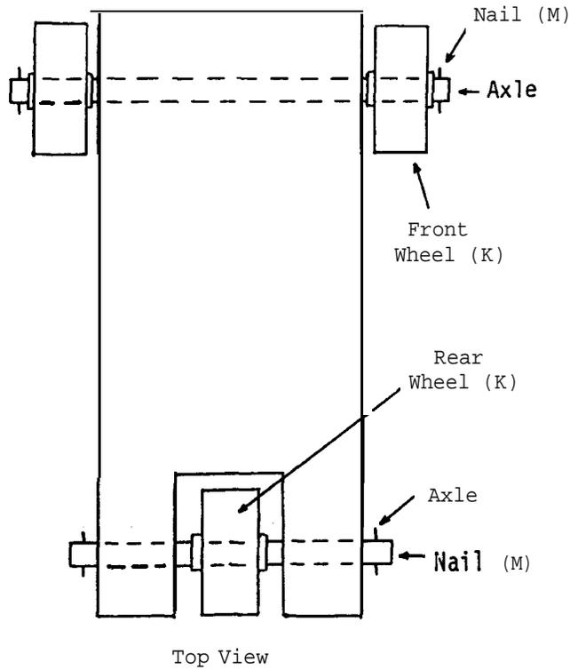
cart. Cut two axles from the wooden dowel (L). Make the front axle 13 cm, and rear 9 cm long (both 0.5 cm in diameter in this instance). The diameter of the dowel should be the same as the internal diameter of the ball bearing wheels, thus providing a tight fit.
