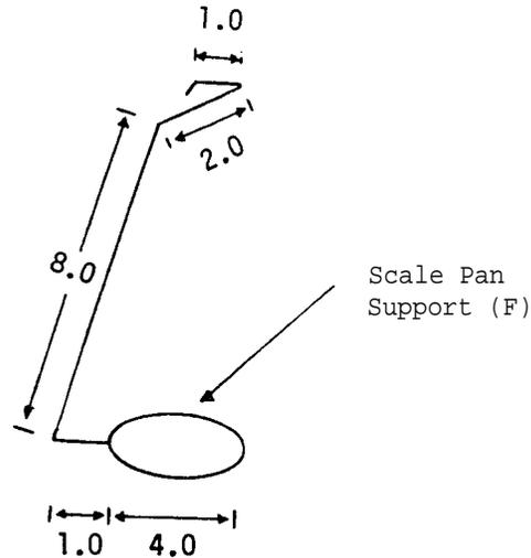
Fold one loop on top of the other, and then bend the remaining straight portion of the wire to the shape indicated. You now have a scale pan support which may be attached to the spring lever.
