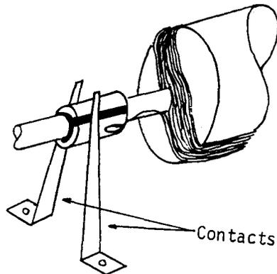
The axle may be held firmly in position by winding masking tape (J) (not scotch tape) around the axle next to, and just outside, the supports. Do this as a last step in constructing this item, however,
