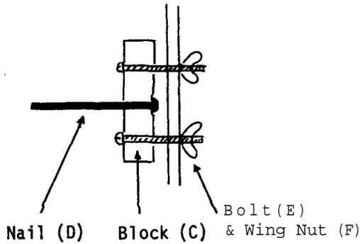
Drill two more holes (diameter 0.3 cm) through the wood, close to the edges, and use bolts (E) and wing nuts (F) to attach the block to the pegboard support stand. The newly attached pivot nail should be at the center of the pegboard and about 20 cm above the base.
