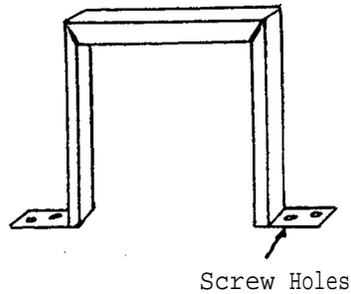
Use galvanized iron or aluminum sheeting (I) to make the vertical support. Cut it to the dimensions indicated, and bend it to the shape of a bridge. Drill two holes (diameter 0.3 cm) in either foot of the bridge so that the support may subsequently be attached to a base with screws.
