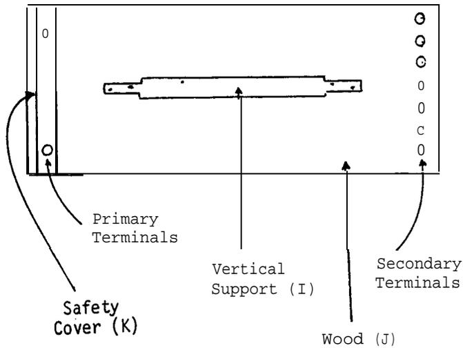
Make a base for the transformer out of wood (J). Fit the vertical support snugly over the core and coils, and attach the support to the middle of the base with screws.
