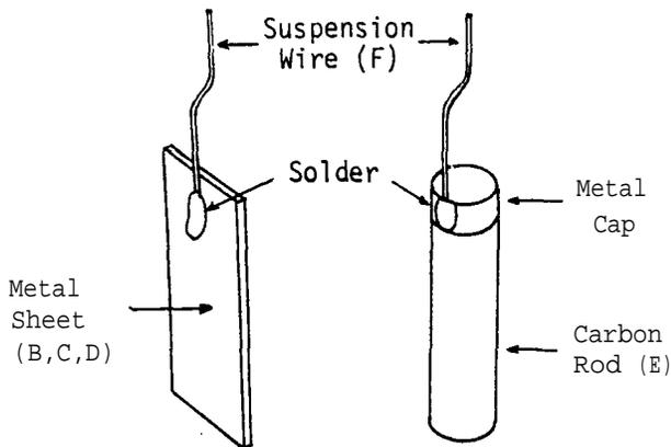
Solder a brass suspension wire (F) on to each of the metal sheets (B, C and D). Also solder a similar suspension wire (F) to the metal cap on a carbon rod (E) extracted from a dry cell.
