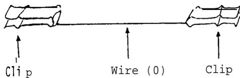
Remove any paint or coating from the wires (M) with sandpaper. Bend one end of each wire into a loop, and slip this onto one of the terminals. Bend the free end of the wire around an adjacent terminal so as to form a spring catch. Make a small lip on the end of the catch, thus permitting the catch to be readily attached to, or released from, an adjoining terminal.
