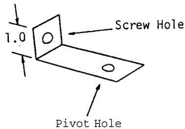
Bend the strip of brass (Q) to form an "L" shape. Drill a screw hole (diameter 0.3 cm) in the short end and a pivot hole (diameter 0.2 cm) at a distance of 0.5 cm from the other end. Slide the strip over the pivot needle, and screw the strip to the upright, with the screw (R).
