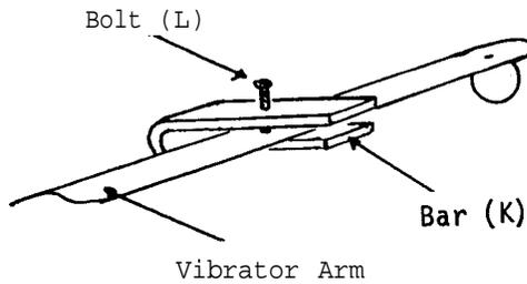
The soft iron bar (K) should weigh approximately 50 g. Place the bar in a strong clamp, and use a hammer to bend it in half so that it becomes two parallel bars about 0.3 cm apart. Drill a hole (0.2 cm diameter) in the middle of the top bar, and make a thread (0.2 cm diameter) in the hole. Screw bolt (L) into the hole thus making it possible to clamp the bar onto the ripple tank's vibrator arm.
