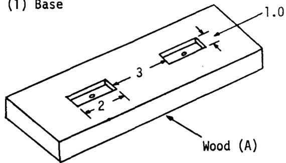
Make two insets (0.5 cm deep) in the wood (A) to take the two uprights (B). Drill a small hole (0.2 cm diameter) in the middle of each inset.
