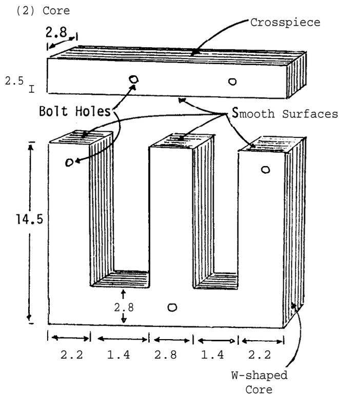
Stack the galvanized iron sheets (E) on top of the other until the pile is 2.8 cm thick. This will require 55, or more, plates, dependent on the thickness of the sheet. Then cut each of the sheets as illustrated to form a W-shaped plate and a rectangular crosspiece.
