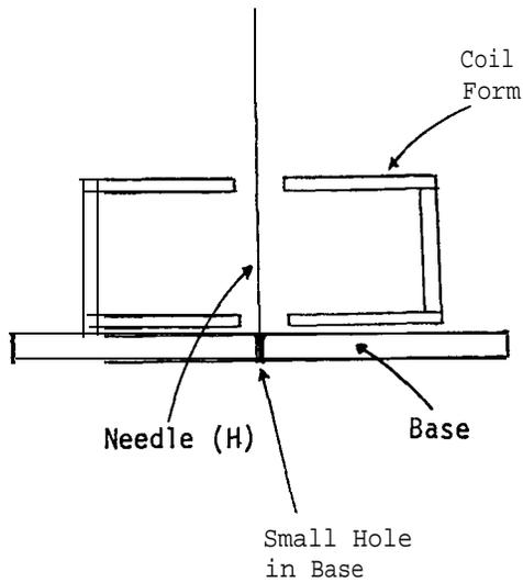
Drill a hole (0.1 cm diameter) in the base in the position that corresponds to center of the larger hole in the base of the coil form. Cut the end (containing the eye) off needle (H) to make it 8 cm long, and set the blunt end of the needle firmly in the hole in the base, so that it stands vertically with the point upwards. A little epoxy resin may be required to hold the needle firmly in the hole.
