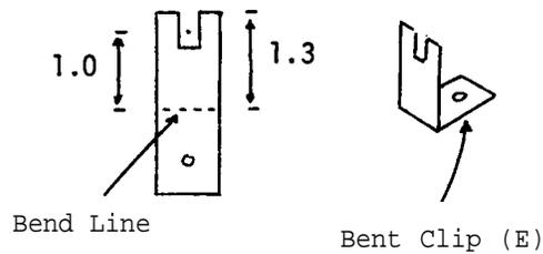
Cut a slot (0.7 cm x 0.3 cm) in the end of each of the brass sheets (E) and drill a screw hole in the other end, thus producing four clip holders.
