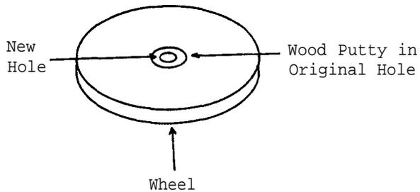
Cut two lengths of wire (0) from wire coat hangers to serve as axles for the cart. Drill holes, slightly less than 0.2 cm in diameter, through the exact center of each wheel, and put a little epoxy resin in the holes.
