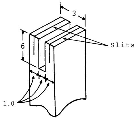
razor blade (F) in half, and, after smearing the cutting edges with epoxy resin, insert the cutting edges of the blades as deep as possible into the slits. The less the blades protrude above the wood the less the strain that is possible on the projecting blades.
