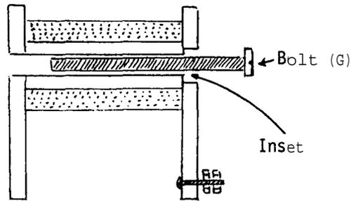
Drill an inset (0.4 cm deep, 1.0 cm diameter) over the hole in the endpiece which contains the terminals. Insert bolt (G) in that the bolthead sits snugly in the inset.
