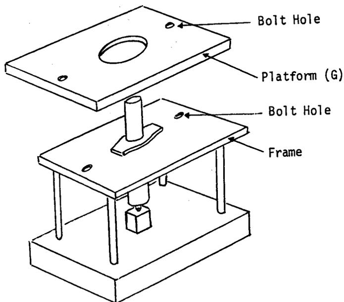
Make the upper platform from wood (G) to fit on top of the existing platform for the frame.
