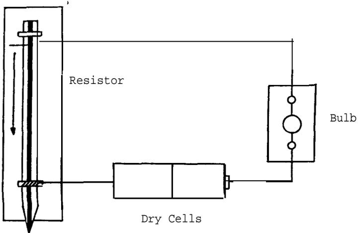
(1.5 volts each) and a flash-light bulb (approximately 1.5 volts), it will be found that increasing the length of pencil lead included in the circuit will diminish the brightness of the bulb, the **full length** of lead (approximately 20 cm of #2B lead) almost extinguishing the light altogether.
