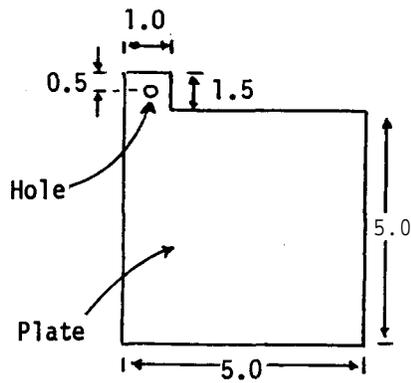
Cut a plate out of lead sheeting (H) and another out of aluminum sheeting (I) to the dimensions shown. Drill a hole (0.3 cm diameter) in the projecting portion of each plate.
