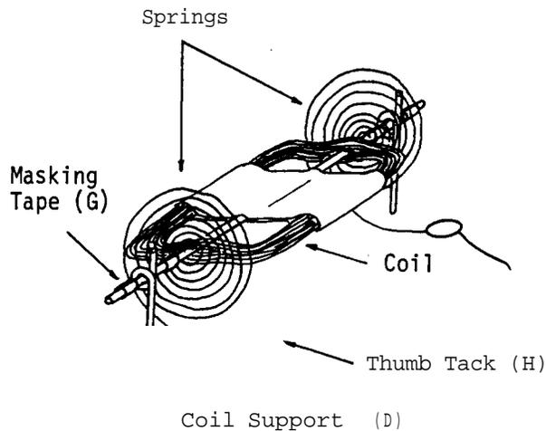
Fit the coil (F) into the coil supports (D) on the base. Wind the 100 cm of magnet wire (E) at either end of the coil into a spring, and attach the wire, just beneath each spring, to the base with the help of a thumb-tack (H). Each spring should contain about eight turns and be about 3 cm in diameter.
