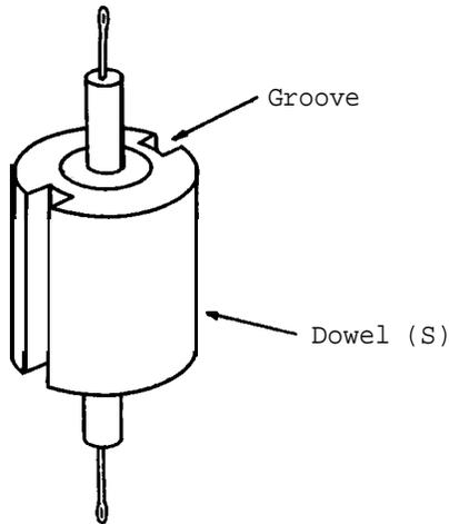
Cut a groove (0.5 cm deep, 1 cm wide) around the wooden dowel (S) to hold the subsequent magnet wire coil in position. Drill a hole (1.2 cm diameter) along the axis of the spool, and insert the newly made stack of washers on the dowel (Q). Use epoxy resin to hold this firmly in position within the dowel.
