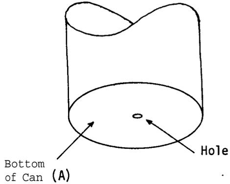
Take ~~the~~ tin can (A) and drill a small hole (0.1 cm diameter for example) in the middle of the base.
