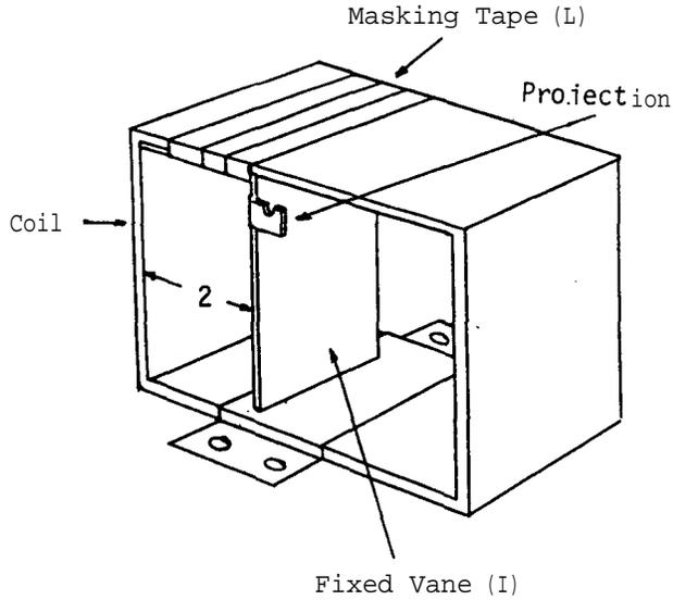
The completed vane may then be fixed vertically in position within the coil by wrapping masking tape (L) around the top of the coil, covering the horizontal portion of the fixed vane in the process.
