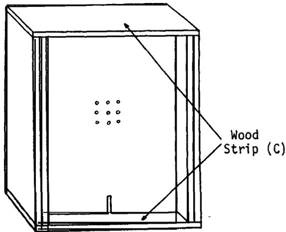
Nail the top and bottom pieces (D) to the two upright pieces to complete the framework. The thickness of the bottom strip (D) should not be much more than 0.5 cm, as there is a tendency for this strip to cut off a desirable portion of any light path.
