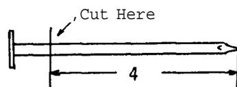
Take a handful of nails (C) and cut off the top ends to produce a uniform set of nails, each 4 cm long. Tap the nails into the bottom strip (A), positioning them in the indentations. Then press the upper strip (A) onto the upright nails, using the indentations on the upper strip for guidance in positioning the nails parallel to one another. Finally, attach the sidepieces (B) of the framework using very small nails or wood cement.
