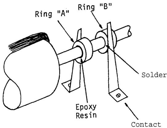
Temporarily remove the axle support and slide the two rings onto the axle. Coat a length of axle (0.5 cm long) with epoxy resin about 0.1 cm thick and slide ring "A" into position over this. The epoxy
