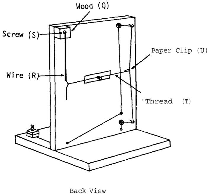
Attach the small wood block (Q) to the rear of the support at the top left-hand corner. Insert a screw (S) into the block and fasten the end of a length of steel wire (R) between the screw and block so that the wire is held rigidly in a vertical position, thus serving as a spring.
