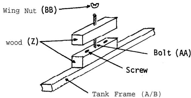
Make the vibrator clamp from two strips of wood (Z). Drill a hole (0.4 cm diameter) through the lower strip, and then attach the strip to the frame with two screws. Set the top strip on top of the first, and fasten it in position with the bolt (AA) and wing nut (BB). The vibrator arms may now be clamped firmly between the strips of the clamp, being held at the middle of the arms. This insures the maximum possible period of vibration.
