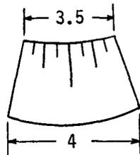
Make a small scale from a piece of white paper (M) by marking regular divisions (0.3 cm apart approximately) on the paper. Glue the scale to the support just behind the pointer so that when the balance arm is perfectly horizontal the pointer will be at the middle of the scale.
