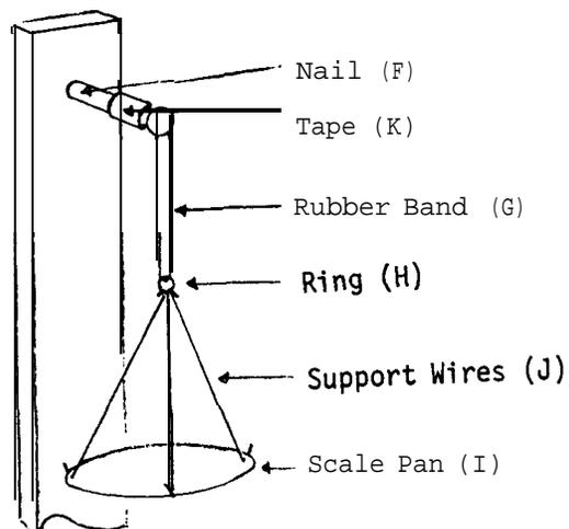
Drive nail (F) horizontally into top of the vertical support, and suspend a rubber band (G) from its end. Take the galvanized wire (H) and bend it into the shape of a ring which can be suspended from the rubber band.
