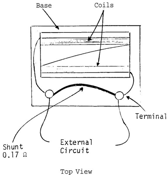
Take a suitable length of nichrome wire (0) and connect it across the galvanometer terminals. In this case, since the resistance of the galvanometer is 1.5 ohms a wire of resistance 0.17 ohms (5 cm of #24, U.S. Standard Plate gauge, nichrome wire, 20% chrome, 80% nickel) would result in 1000 milliamps (1 amp) producing a full scale deflection instead of 100 milliamps doing this.
