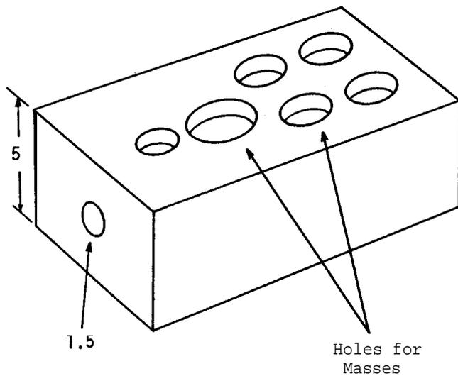
Bore a hole from the center of one end of wood (A) to the center of the other end, in order to accommodate a spring device. The diameter of the hole (1.5 cm) should be slightly larger than that of the spring (1.2 cm).
