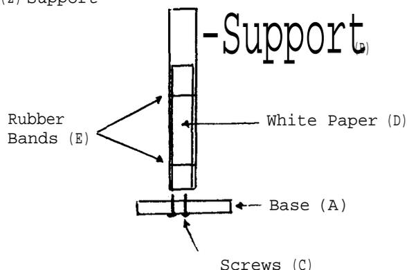
Attach wood strip (B) vertically to the base with two screws (C). Attach the plain white paper (D) to the front of the vertical support (B) with rubber bands (E).
