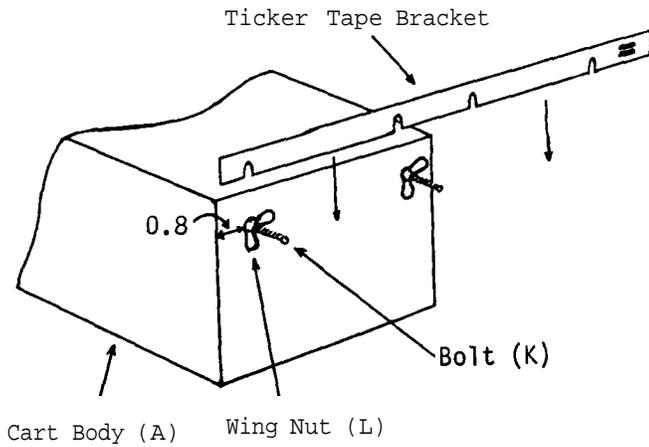
rear of the cart. Wing nuts (L) should be used to fasten the bracket in position.
