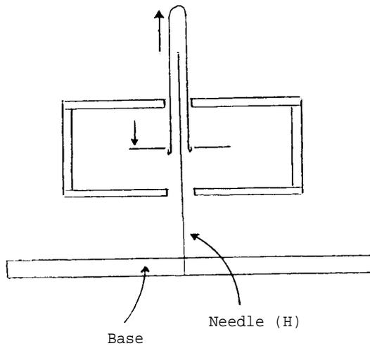
Lower the blade onto the flanges of the glass tube, and raise the tube partially through the upper hole in the form.
