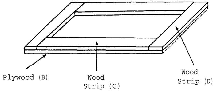
Make the base from the piece of plywood (B). Nail the two short pieces of wood (D) to the ends of the plywood (B) and nail the remaining wood strips (C) to the plywood, too. Make sure that they will hold the lamp housing firmly in position. Then nail it into position.
