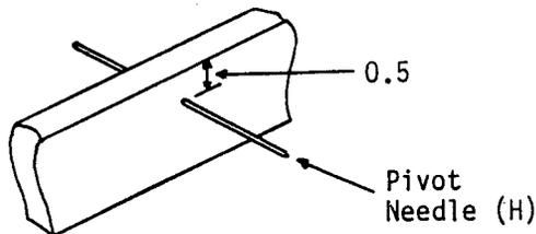
Drill a hole (0.1 cm diameter) horizontally through the middle of the arm at a distance of 0.5 cm from the top of the arm. Drive the steel needle (H) through the hole to serve as a pivot, and glue it permanently in position with epoxy resin.
