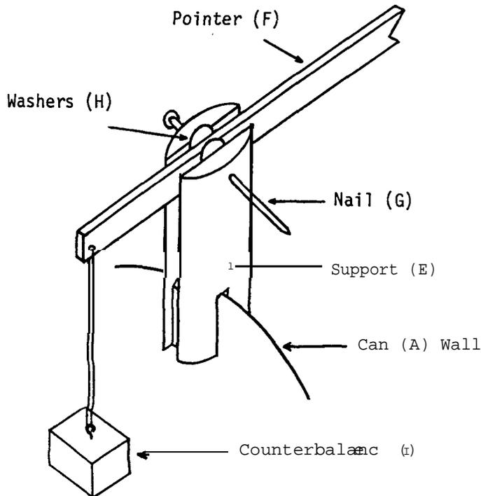
Balance the pointer on the newly made support by inserting the nail (G) through the appropriate holes in the support and pointer. Washers (H) should be placed either side of the pointer to serve as spacers. These prevent unwanted motion of the pointer on the pivot. The pivot may be fixed permanently in position in the support with the help of epoxy resin, since the pointer can move about the fixed axle on its own pivot hole.
