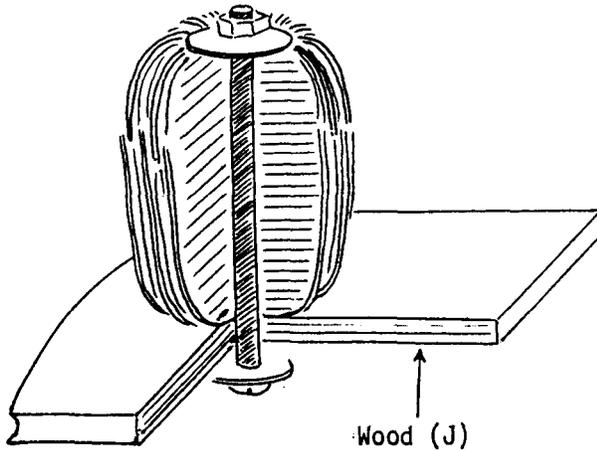
Make the base from wood (J). Drill a hole (diameter 0.5 cm) through the center, and attach the coil and core to the base with the help of the bolt (G) through the middle of the core. Make an inset in the bottom of the base to accommodate the bolt-head.
