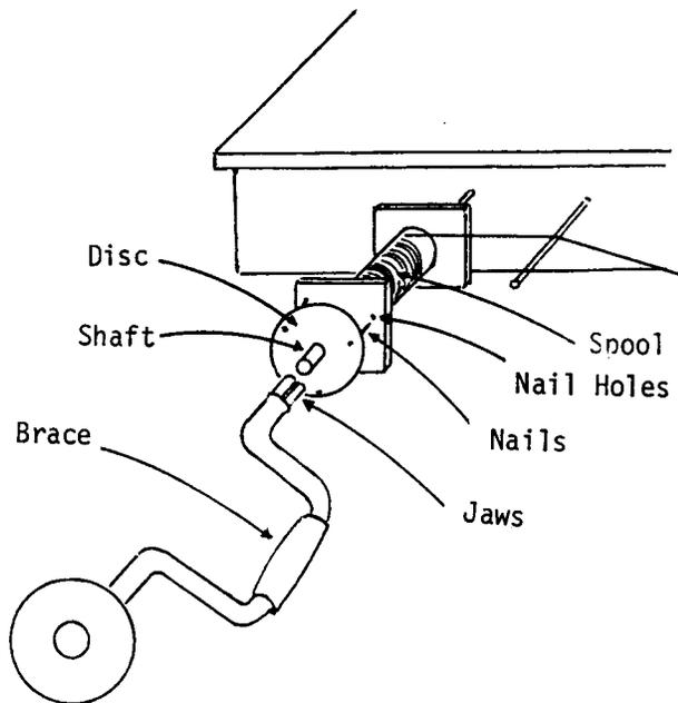
Hammer two large nails (15 cm long) into the side of a bench so that they protrude horizontally some 50 cm apart. Place the spool to be wound on one of the nails. Fasten the first turn of magnet wire around the spool in such a way that it will not slip on turning the spool. Then get your partner to hold the wire taut over the second nail so that it may be wound under tension.
