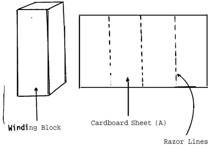
Cut a piece of wood (10 cm x 3 cm x 3 cm) to serve as a winding block for the primary and secondary coils. Take the sheet of cardboard (A) and use a razor blade to score parallel lines on it at 3 cm intervals so that it may readily be bent to the shape of the wooden block.
