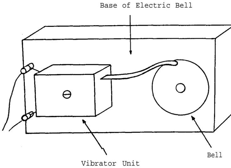
Take the household electric bell (A), and remove the vibrator unit. (The bell utilized in this instance was designed to operate normally at 10 volts.)
