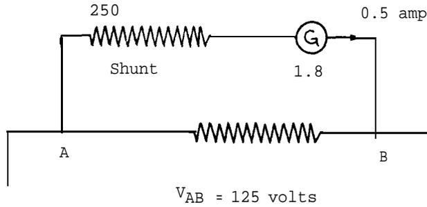
used as a voltmeter, the full-scale deflection corresponding to 125 volts (DC). One way of conveniently doing this is to add a third terminal [see VIII/A2, component (4)] to the front of the galvanometer base, simply placing the shunt (obtained from a radio shop) across two adjacent terminals.
