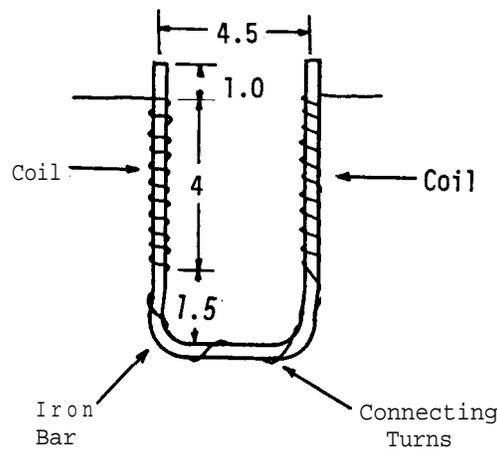
connecting turns. The coils may be held in position by means of masking tape. If the coil is connected in series into a separate electrical circuit, it may be used in precisely the same way as the former horseshoe magnet.
