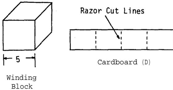
Cut a piece of wood (5 cm x 5 cm x 5 cm) to serve as a winding block for the coil. Use a razor blade to score parallel lines on the cardboard (D) at 5 cm intervals so that it may be readily bent into the shape of the wooden block.
