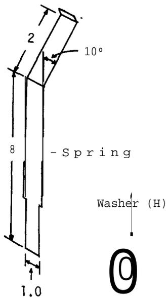
Cut the packing case band (G) as indicated to make the spring. To facilitate the throwing of the washers (H) by the spring, bend the top end of the packing case band at an angle. Insert the spring through the remaining slits in the cart.
