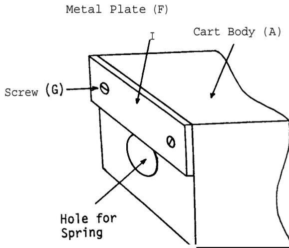
Fasten the metal plate (F) (brass, steel, etc.) onto the front of the cart with two screws (G) so as to just overlap the top of the hole for the spring.
