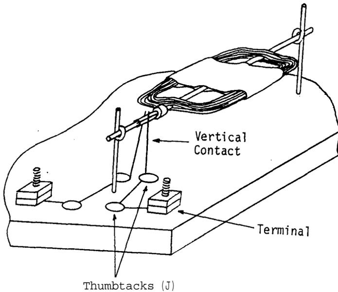
Take the length of straight coat hanger wire (F) and thread it through the middle of the coil to serve as the axle. Wrap the masking tape (H) around the coil and axle to hold the coil firmly in position.
