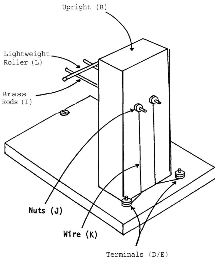
Drill two horizontal holes (0.4 cm diameter) through the upright (B). It is important that the two holes should be at exactly the same height (6 cm) above the base, and that they should be perfectly horizontal.
