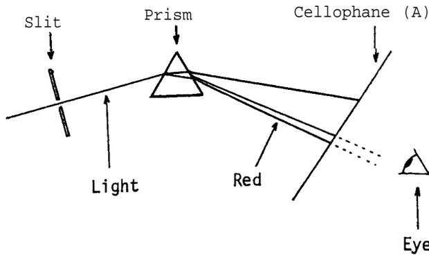
Test different strips of red cellophane (A) for suitability by noting what parts of a spectrum can be seen through the cellophane. The cellophane cutting out almost all colors other than red will be most suitable.
