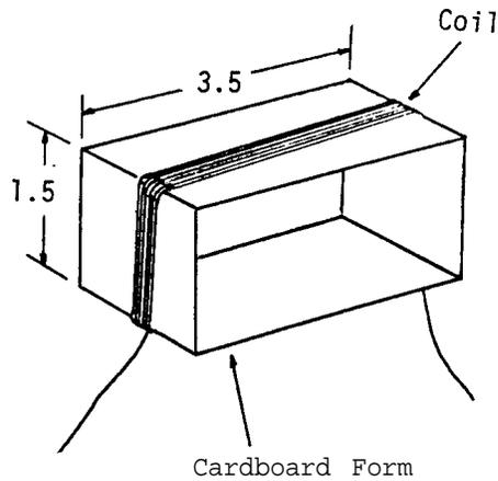
Wind 30 turns of magnet wire (E) around a cardboard form in order to make a coil of internal size 3.5 cm x 1.5 cm. Leave 100 cm of wire free at either end of the coil.
