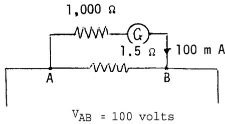
Without a resistance in series, the full-scale deflection of the galvanometer would only measure 0.15 volts across the terminals. With the 1,000 ohm resistance in series, the full-scale deflection of the galvanometer would measure 100 volts across the terminals. More important, the current taken through the galvanometer, compared with that in the circuit being measured, would be negligible.
