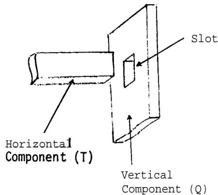
Cut a rectangular slot (2 cm x 1 cm) in the top of wood (Q) to take the horizontal component, wood (T). Fasten the two firmly together with wood cement. Glue a triangular piece of wood (U) between the two components to make a stronger junction.
