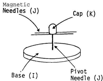
Use the wood disc (I) as the base of the compass. Alternatively, a cork disc would serve equally well, although less durable.
