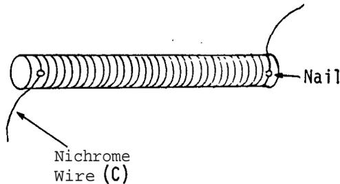
The dimensions of the apparatus depend very much on the resistance required. In this case a 25 ohm resistor, capable of carrying a current of up to 3 amps was required, and it was decided that this could be achieved by using some 400 cm of #20 nichrome wire which had a resistance of approximately 1 ohm per 16 cm length. This determined the dimensions of the coil and the resulting item of equipment.
