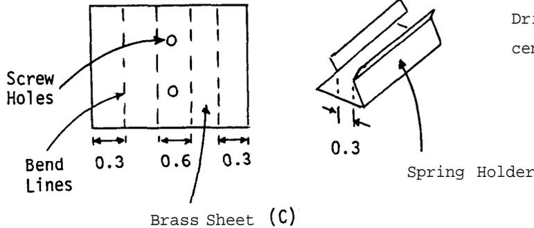
Bend the two brass sheets (C) into spring holders as indicated. Drill two screw holes in the center portion.
