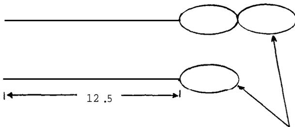
Take the galvanized iron wire (F) and make it into a double strand 25 cm long. Use half of the new length to form a "figure 8" in the wire.
