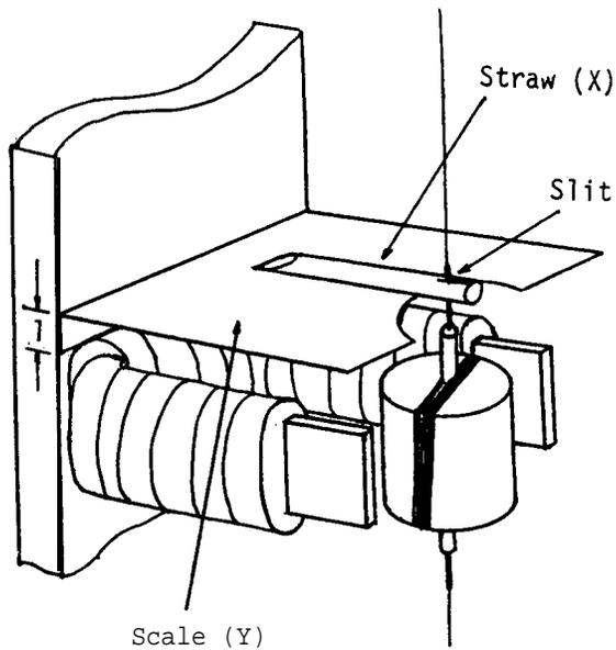
A pointer for the galvanometer may be made from a soda straw (X). Make a small slit in the end, and fit it around the eye of the needle at the top of the dowel (S). A little glue will hold it firmly in position.
