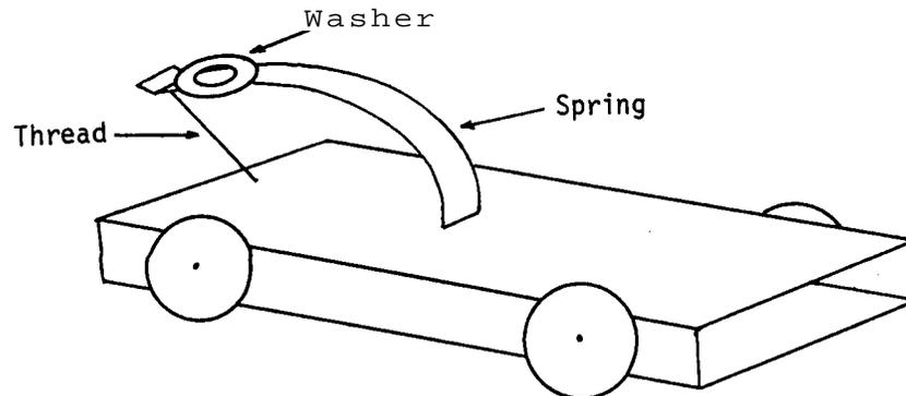
match is applied to the thread, the spring will be released and eject the washer forward, while the cart will be propelled backwards, thus offering another demonstration of action and reaction.
