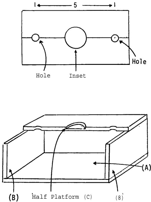
Make a four-sided wooden support from the wooden base (A), wooden sides (B) and platform (C). Fasten the base and sides together with small screws (D) and wood cement, but do not put the platform in position yet.
