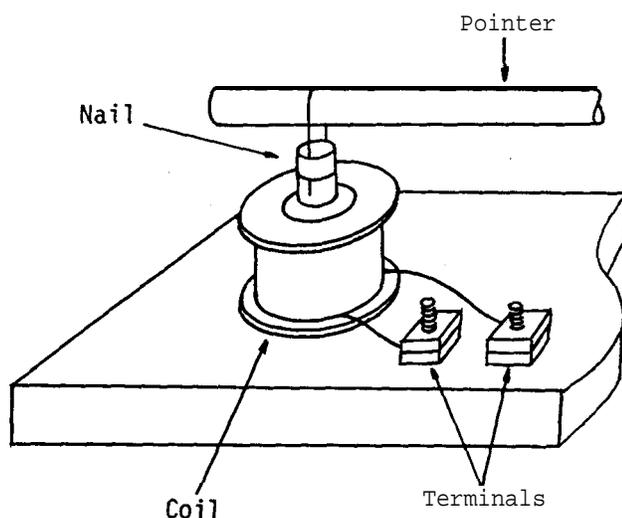
Wind the magnet wire (M) onto the paper cylinder to make a coil. Leave 10 cm of wire free at either end. Cover the last layer of wire with masking tape (N) to hold the coil in position. Remove the coil from the dowel, and mount it on the end of the base with glue in such a way that the axis of the coil is directly beneath the nail suspended from the end of the straw balance arm.
