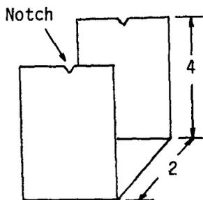
Using a small file cut a shallow, smooth notch in the top of each side of the support to hold a subsequent needle pivot in position.
