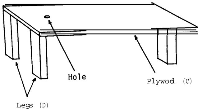
Take plywood (C) to make the platform, balancing this on the three leg (D) which should be sufficiently long to permit the lower reservoir to be moved under the platform without difficulty. Drill a hole (1 cm diameter) in one end of the platform. Place the upper reservoir over the hole in the platform and the lower reservoir underneath it so that water can run from the upper to lower reservoir.
