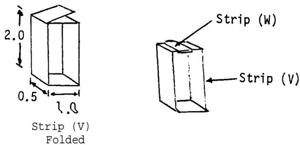
In order to attach the lamp housing to the horizontal components of the support make two brackets from steel strips (V) as illustrated. Cut four horizontal slots in the upper part of the lamp housing and
