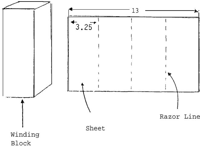
Cut a piece of wood (14 cm x 3.2 cm x 3.2 cm) to serve as a winding block for the primary and secondary coils. Take the thin sheet of cardboard (A) and use a razor blade to score parallel lines on it at intervals of 3.25 cm, so that the cardboard may readily be bent around the wooden block.
