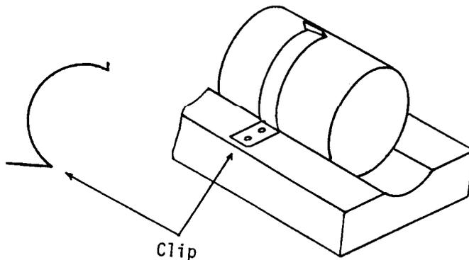
However, should any problem occur (e.g., due to bad alignment of the adjustment screw) the cells could be held more firmly in place by means of clips made from packing case bands.
