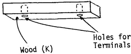
In addition, make a safety cover for the primary terminals from wood (K). Simply cut holes (2 cm deep, 1 cm diameter) in the undersurface to accommodate the terminals, and set the wood on the base so that it covers the terminals.
