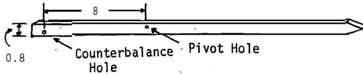
Make the pointer from a strip of wood, (F). Drill a small hole (0.3 cm diameter) at one end of the pointer to take the string (J) from the counterbalance, and 8 cm away from this hole drill a second hole (0.3 cm diameter), close to the top surface of the pointer, through which the nail (G) is to be put as a pivot.
