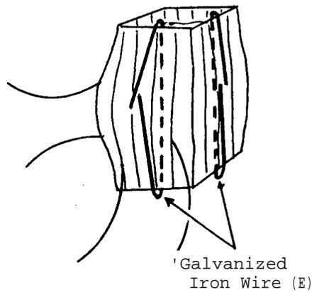
Take the dry wires one at a time, and bend them through, and around, the coil so that the wire ends just touch, or overlap, one another. If the wire is too long, cut the ends. Continue adding the iron wires to the coil in the same way, distributing the wires equally on each face of the coil, until the coil is almost full of iron wire. However, leave enough space to squeeze bolt (G) through the middle of the wire core.
