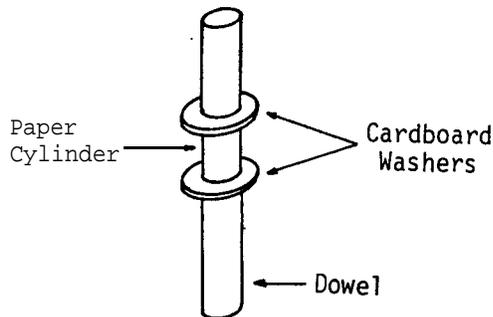
Cut two washers (internal diameter 1.0 cm, external diameter 2.0 cm) from the sheets of cardboard (L). Attach the washers to the ends of the paper cylinder with glue.
