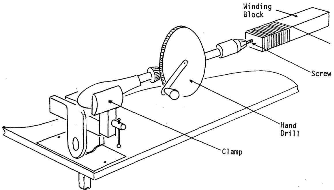
(i) A convenient way of winding the coils is to use a hand drill and winding block. Clamp the hand drill horizontally above the bench surface, and hold winding block horizontally in the drill chuck with the help of a screw fixed firmly in the end of the winding block. If a cardboard sleeve is fitted over the winding block, the wire may be wound on the sleeve, and the latter subsequently removed complete with newly wound coil.
