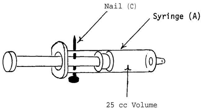
Use a drill of a slightly larger diameter than that of the nails (C) to carefully make holes through the barrel and plunger of the plastic syringe (A). When the nail (C) is inserted through these holes, the plunger should be held in a position such that the volume in the syringe is 25 cc. Similarly, prepare the second syringe (B) so that the volume is held at 5 cc capacity when the nail is in place.
