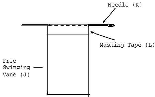
The free swinging vane is made from the other sheet of galvanized iron (J) and suspended from the middle of the needle (K) by wrapping a piece of masking tape (L) over the end of the vane. Suspend the vane from the projections on the fixed vane.
