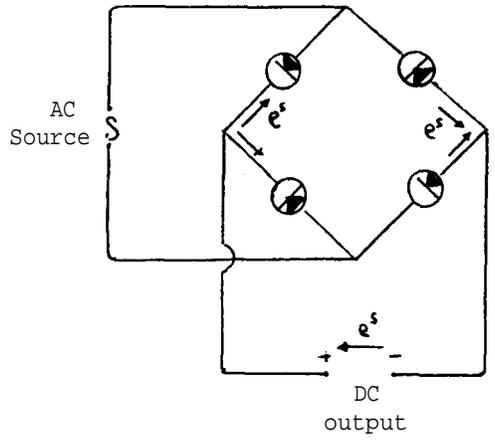
Use copper wire (O) to connect the plates of the four cells together, as indicated in the diagram. The cells have the simple property of permitting electrons to flow only in one direction, from aluminum to lead, and when connected as indicated to an AC source a rectified output is obtained. The type of output obtained with AC sources of 12 volts and 25 volts is indicated in the notes.
