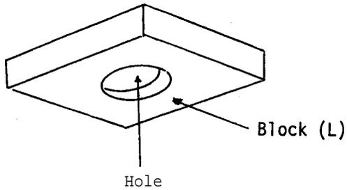
Take the wooden block (L), and drill a hole (the same diameter as the plunger, and 1.5 cm deep) into the middle of the block. Nail the scale pan squarely on to the undrilled surface of the block. Line the inside of the hole in the lower surface with wood filler.
