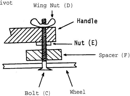
Use the bolt (C) to serve as the pivot for the wheel. Insert this through the wheel, the spacer (F), a locking nut (E) and the handle (B). Use the locking nut (E) and the wing nut (D) to hold the handle in a fixed position on the pivot,
