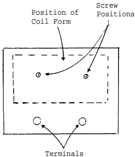
Drill two appropriate holes through the base in order to attach the coil form to the base with screws, but do not screw the form on to the base yet.
