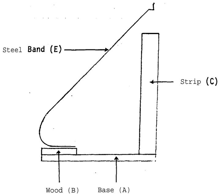
Attach the drilled end of band (E) to the top of block (B) on the base with two small nails. Bend the band smoothly over to form an elongated C-shape as indicated.
