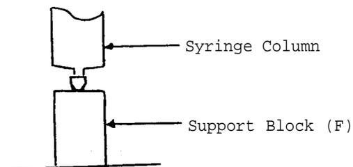
Insert the syringe column through the hole in the platform. It will hang suspended with a gap between the bottom of the syringe and the surface of the base. Cut a small support block (F) to fill this gap, and drill a small inset into the top of the block to hold the syringe firmly in position. (The block will also prevent the modelling clay seal in the bottom of the syringe being readily broken under pressure). Fasten the support block to the base with wood cement.
