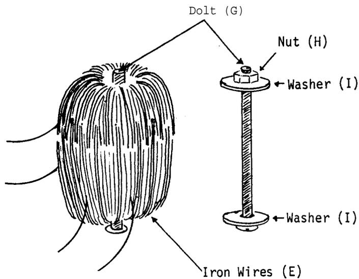
Slide bolt (G) through the middle of the iron wires. Washers (I) should be fitted on either end of the bolt, and the whole kept in position with a suitable nut (H).
