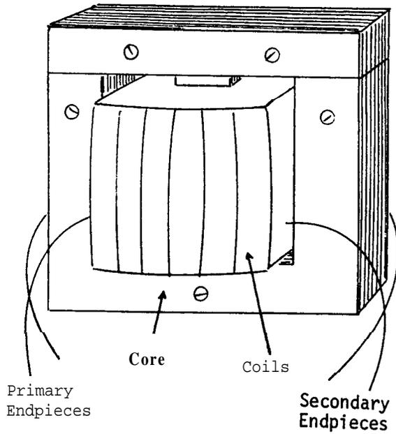
fasten the plates of the cross-piece and core together.
