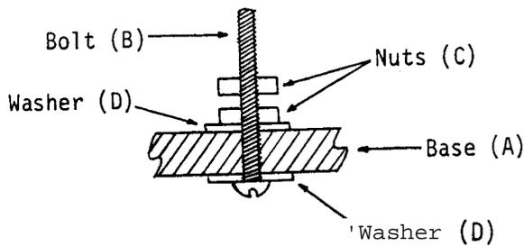
Drill holes (0.4 cm diameter) in the base (A) in the terminal positions, making sure that the holes are at right angles to the plane of the base. Use a bolt (B), two nuts (C), and two washers (D) to make each terminal.
