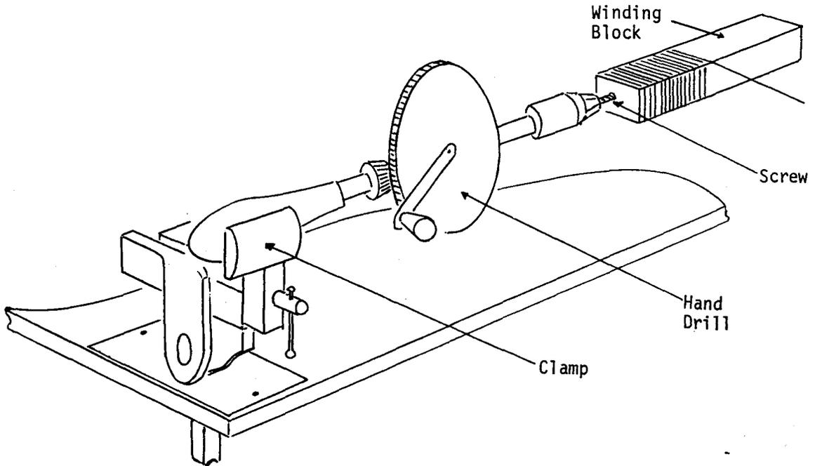
(i) A convenient way of winding the coils is to use a hand drill and winding block. Clamp the hand drill horizontally above the bench surface, and hold a winding block horizontally in the drill chuck with the help of a screw fixed firmly in the end of the winding block. If a cardboard sleeve is fitted over the winding block, the wire may be wound on the sleeve, and the latter subsequently removed complete with newly wound coil.
