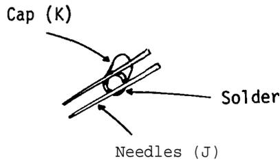
Hold the needles parallel to one another and drop some solder on the base of the cap. Immediately attach the needles (at their centers of gravity) to the cap by placing them in the still molten solder.
