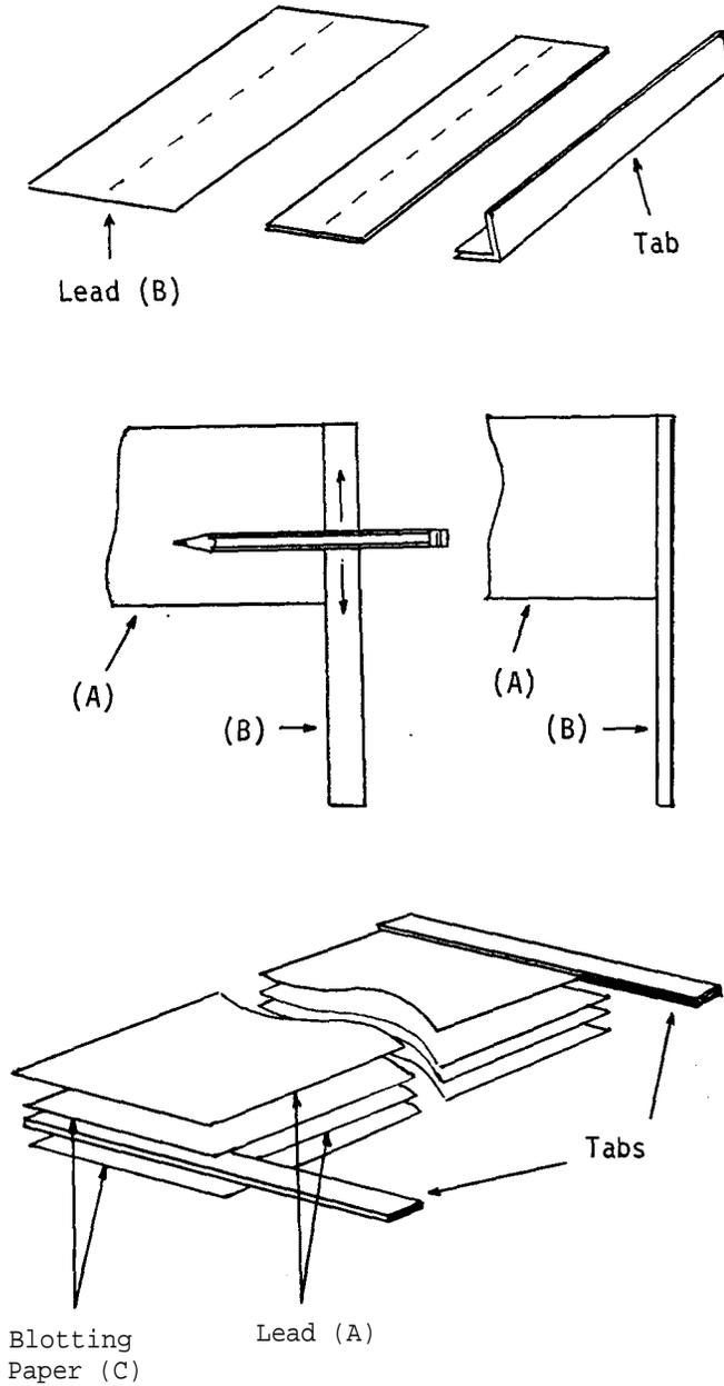
Fold one of the small lead sheets (B) down the middle. Repeat the process again, but this time leave the fold open. You now have a tab for attachment to one of the lead plates.
