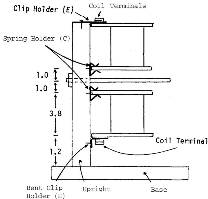
Use screws (D) to attach the spring holders horizontally to the upright of the apparatus, 1 cm above, and 1 cm below, the horizontal rods. Clip the multipurpose coils temporarily in the spring holders, and mark out the positions of the free endpieces of the coils.
