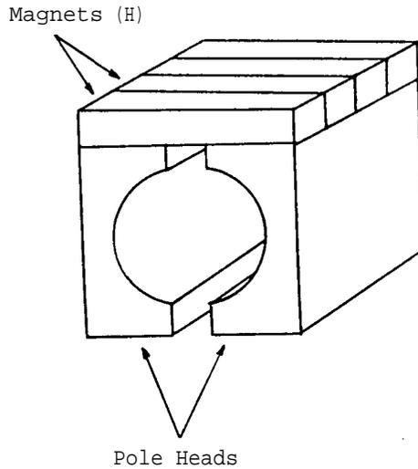
the pole heads. The magnet may be purchased, or made (as described under IX/A) from the steel bars (H).
