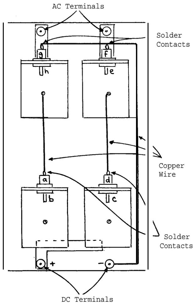
Take the copper wire (H) and connect the silicon diodes as illustrated. It will be necessary to solder the wire on to the ends of the diodes, and particular care should be taken to avoid overheating, since this can destroy the diodes.
