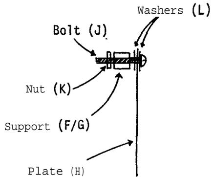
Attach the lead plate to the plate support with the help of bolt (J), nut (K) and washers (L) placed either side of the plate.
