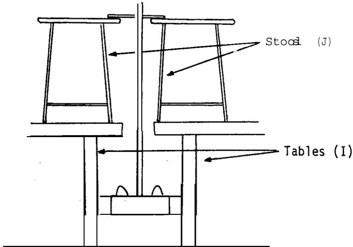
Place two tables (I) fairly close together, and sit the stools (J) on top of both tables, sufficiently close to one another so that the pendulum may be supported by means of its pivot nail resting between the tops of the stools. The nail (G) must be held firmly in position on top of the stools hand, clamps, or any device which will hold it firmly.
