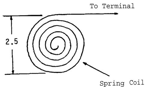
Wind 40 turns of magnet wire (N) around the inset of the core, making sure that both ends are left free. Clean the ends of the wire with sandpaper and solder each end on to another length of very fine magnet wire (O) from which fine spring coils may be made around the top and bottom portions of the pivot.
