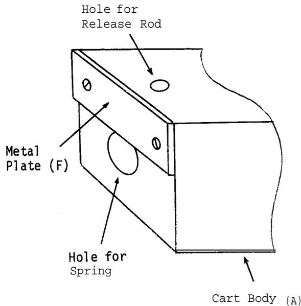
Bore a vertical hole (diameter 0.5 cm) into the top of the cart, near the front end, so that it meets the horizontal bore hole for the spring. The small wooden rod (H) (release rod) inserted into this hole, and pressed against the horizontal rod of the spring device itself, will release the spring from its state of compression. (The need to have the diameter of the spring bore hole slightly
