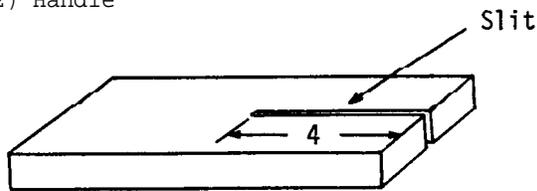
The handle is made from the wood (B). Cut a slit down the middle of the handle with a saw. Cement the metal strip into this inset with epoxy resin.
