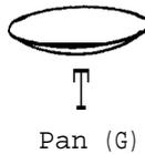
Make the pan itself from the aluminum sheet (G). Hammer it at the center to create a saucer shaped pan. Sit the pan on the loop of the scale pan support.
