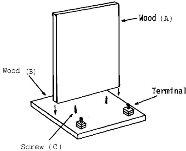
Attach the vertical component (A) to the middle of the base (B) with the help of screws (C) and wood cement.
