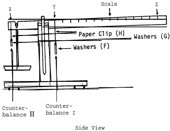
The latter should be such that when it is suspended from the end of the balance arm (position Z) it will just balance the 300 g mass. (In this particular instance two washers weighing a total of 70 g were found to be ideal.)
