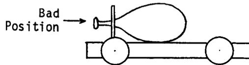
the cart by the expulsion of air. The cart will be accelerated most efficiently if the open end of the balloon is held in such a way as to prevent it flopping from side to side with resultant dissipation of energy in all directions.
