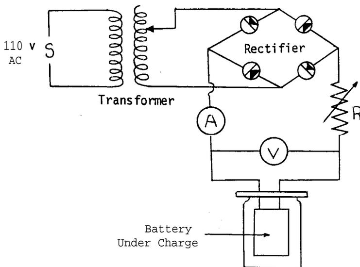
and rectifier (VII/B2) Connect the rectifier to the 10 volt taps on the transformer, and connect the battery across the rectifier as illustrated. A variable resistor (VIII/C2) should be connected into the circuit to control the current, and an ammeter and voltmeter connected as indicated to monitor the circuit.
