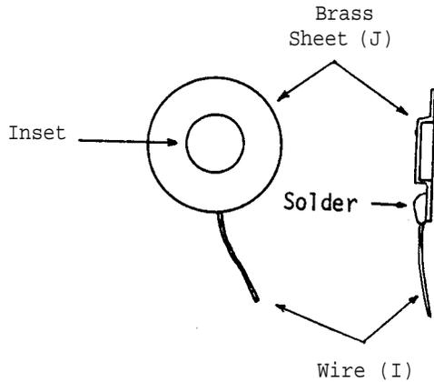
Use a nail head, or punch, to make a central inset (1 cm diameter, 0.2 cm deep) in the two brass sheets (J). Solder the two plates to the bare ends of the wire (I) attached to the two middle terminals. The contact plates are placed between the first and second, and second and third cells, thus enabling the apparatus to provide an external circuit with 1.5, 3.0 or 4.5 volts according to the terminals connected to the circuit.
