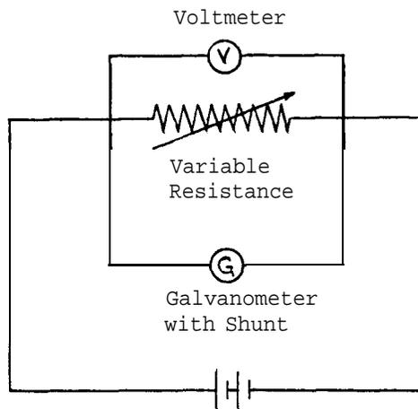
The modified galvanometer may then be calibrated by placing it in parallel across a variable resistance, and comparing the potential at any moment with that indicated by a commercial voltmeter, also placed in parallel across the variable resistance.
