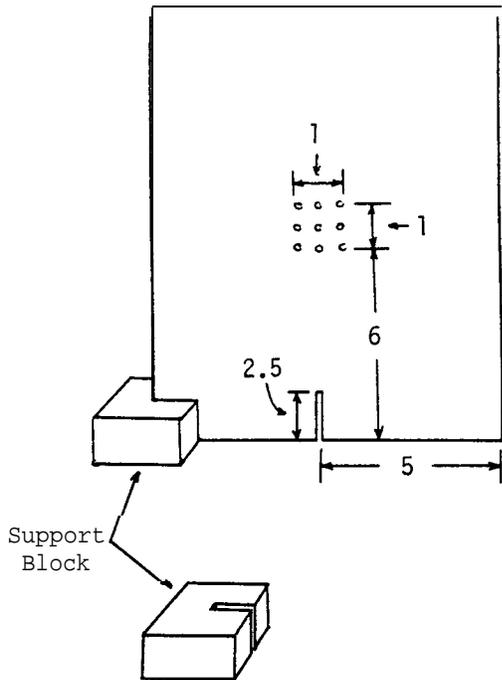
Cut the slit (0.1 cm width) and apertures (0.1 cm diameter) in any suitable thin sheeting (A) (metal, bakelite, cardboard) so long as the slit and apertures have clean cut edges. If the material used is relatively rigid, a small wooden block will provide adequate support. If the material tends to flex under its own weight, a framework, such as that indicated below, will be required for support.
