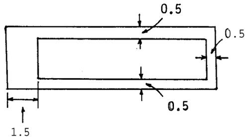
Cut the two pieces of cardboard (B) to the shape indicated, and stick (or clip) a suitable piece of red cellophane (A) between the two pieces.
