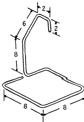
Take the length of aluminum or galvanized wire (K) and bend it into a support for the scale pan. Make an identical support in the same way, and suspend both supports from the notches in the balance arm,
