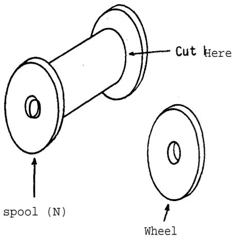
Cut the four wheels from the ends of two wooden spools (N). Fill the spool holes with wood putty and allow the putty to dry hard.
