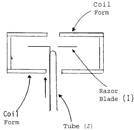
To put the magnetic needle assembly together, hold the razor blade horizontally inside the coil form. Insert the glass tube through the base hole in the form, and then through the hole in the blade.
