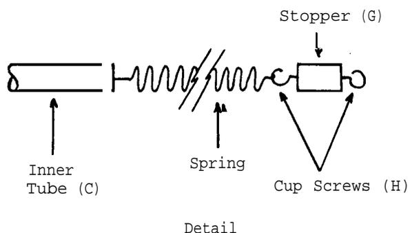
Make a wooden stopper (G) to fit one end of the hollow aluminum tube (F). Fix cup screws (H) in either end of the stopper, and attach the top of the spring to one of the cup screws,
