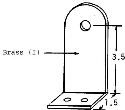
Make two axle supports out of the two brass sheets (I), drilling one hole (0.8 cm diameter) in the upright portion to take the axle, and two holes (0.3 cm diameter) in the base portion to take two screws.
