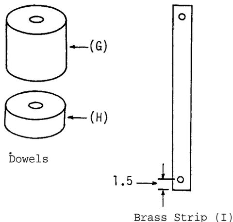
Bore a hole (diameter 0.3 cm) along the axis of each dowel (G,H). Similarly, drill a hole (0.3 cm diameter) at a distance of 1.5 cm from either end of the brass strip (I).
