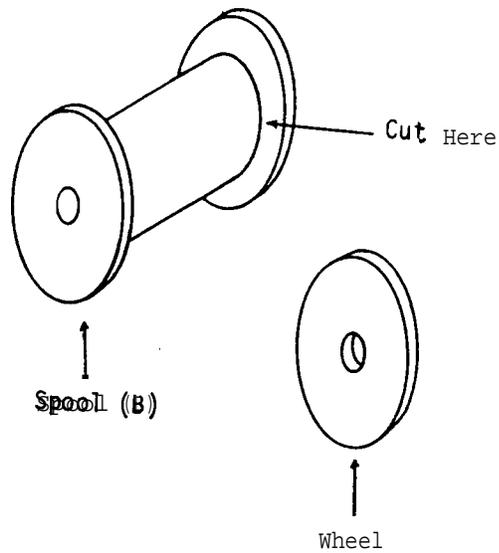
Cut the four wheels from the ends of the two wooden spools (B). Fill the spool holes (0.5 cm diameter) with wood putty and allow the putty to dry hard.
