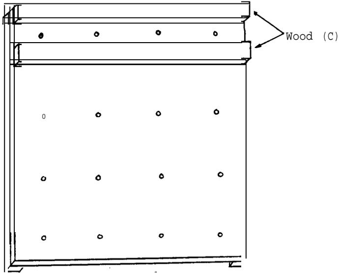
Use two pieces of wood (C) to serve as the cell holder strips. Using nails and glue attach one strip to the end of the base which has not yet been drilled with holes. Place the second strip parallel to, and about 3 cm away from, the first strip. Adjust the separation between the two strips so that they will hold three dry cells (D) snugly in position. Then glue and nail the second strip firmly in position.
