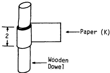
Wrap the paper (K) around a wooden dowel (1.0 cm diameter) to make a paper cylinder. Secure the loose ends of the paper with masking tape (N).
