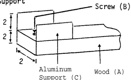
Bend the aluminum sheet (C) into a three sided support. Drill a hole (0.2 cm diameter) through the middle of the support base, and then attach the support to the end of wood (A) by means of a screw
