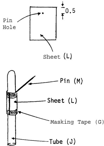
Take the thin sheet of cardboard (L), and thrust pin (M) through the sheet at about 0.5 cm from the middle of the top edge. Bend the cardboard around the glass tube (J) to form a tight cylinder from which the full length of the pin will protrude. Fasten the free ends of the cardboard sheet together with masking tape wrapped around the cylindrical sheet.
