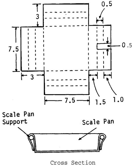
Make the scale pan from the sheet of aluminum (L). Cut squares (3 cm x 3 cm) from the sheet corners to make four projections on the sheet, and cut a slit in one of the projections as indicated. Fold the projections along the dotted lines converting the aluminum sheet into a scale pan with sides. Sit the scale pan on the framework of one of the support wires. Make a second scale pan in an identical manner.
