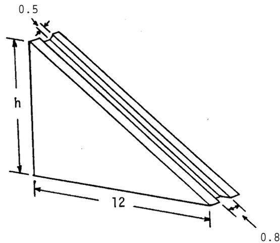
Cut two triangular shapes out of the pieces of wood (D,E). The height (h) of one triangular shape will be 5 cm and the other will be 3 cm, while both will have a base 12 cm long.
