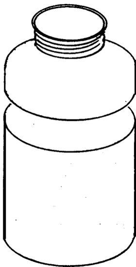
To make a cell container, take jar (A), and use a hot nichrome wire (CHEM/I/F2) to cut the top off the jar some 6 cm above the base. Repeat the process with three more jars.
