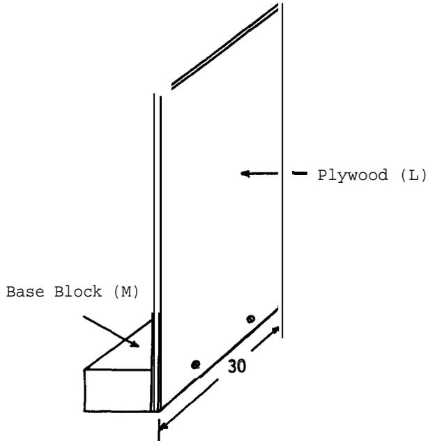
Attach a sheet of plywood (L) to the block of wood (M) intended to hold the plywood in a vertical position. Sit the newly made scale on the platform just behind the end of the pointer, sufficiently close to avoid parallax problems in recording the movement of the pointer. Screw the base block (M) of the scale onto the platform. Use a white sheet of paper (N) attached to the surface of the plywood with thumbtacks to actually record a time scale.
