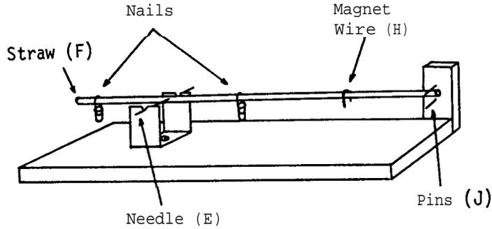
the short nail at the end of the short arm of the straw, and hang the long nail at an appropriate point on the other side of the pivot to serve as a counter-balance. A drop of glue (or a small piece of masking tape) can insure that the loops do not slip along the straw.
