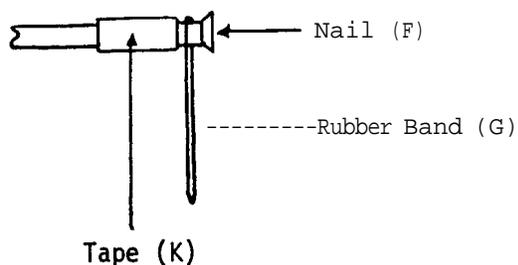
To prevent the rubber band sliding backwards and forwards on the supporting nail a length of adhesive tape (K) should be wrapped around the nail so as to leave a groove between the tape and the end of the nail, the rubber band being held in position in the groove.
