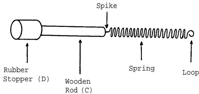
1.2 cm in diameter, and with about 0.5 cm separation between each turn. (A method of winding the spring is described under I/C4). Straighten out one end of the spring into a spike and the other to a horizontal loop. Attach the spring of one end of the wooden rod (C) by means of the spike and epoxy resin. Attach the rubber stopper (D) to the other end of the rod.
