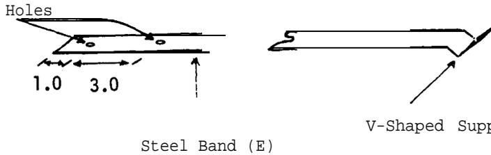
Take packing case steel band (E) and make a small V-shape at one end to hold the scale pan support wire. Drill two holes in the other end to take two small nails.
