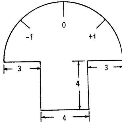
Take the straw (K) and, after piercing it 1 cm from one end, fit it on the end of the axle. A little glue will fix it firmly in position. Cut a suitable scale out of cardboard (L), and attach it to the base, so that it stands just behind the pointer.
