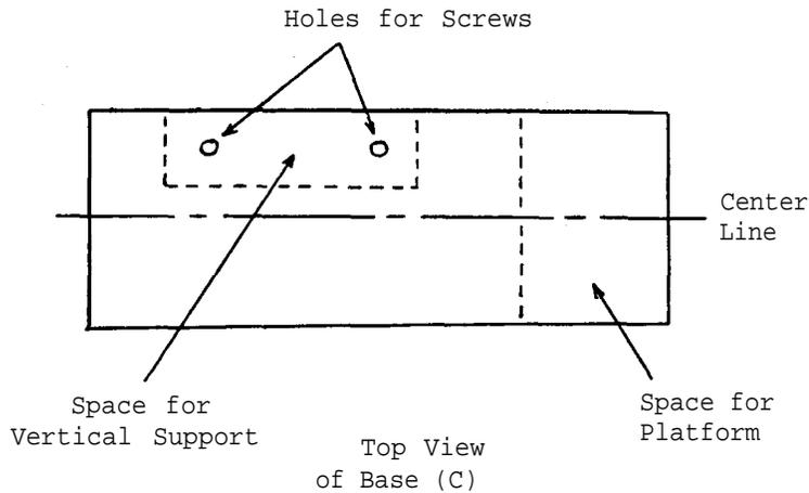
Use the wood piece (C) as the base. Place the vertical support on the base in such a position that the vibrator arm will be parallel to, and directly above, the line bisecting the length of the base. Mark in the position of the support, and then drill two appropriate holes in the base so as to facilitate the attachment of the support with the screws (D).
