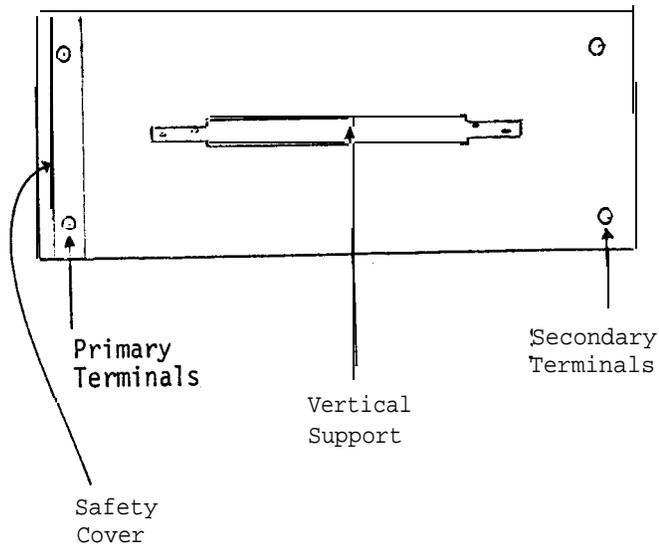
Use galvanized iron or aluminum sheeting (I) to make the vertical support. Cut it to the dimensions indicated, and bend it into the shape of a bridge. Drill two holes (diameter 0.3 cm) in either foot of the bridge so that the support may subsequently be attached to a base with screws.
