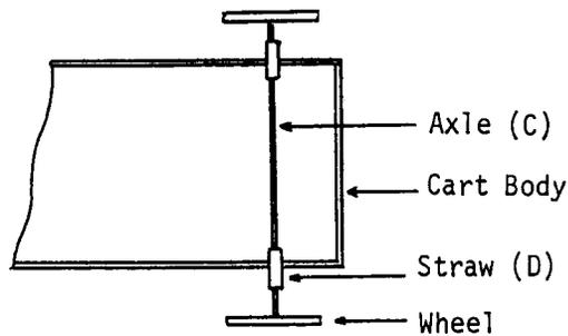
Insert the axle through the body of the cart, and attach a second wheel by the same process. Repeat the procedure with the remaining two wheels and axle, thus providing the cart with front and rear wheels.
