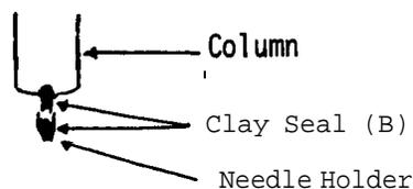
Take the disposable plastic syringe (A) and remove the needle and the top flanges. Remove the plunger from the column, and smear the end of the plunger with petroleum jelly thus insuring a well lubricated plunger, and a good airtight seal.
