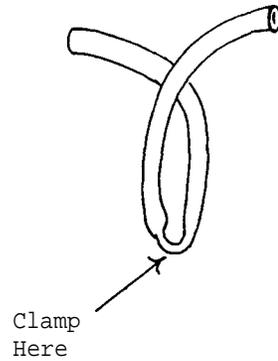
Connect the two syringes with the length of plastic tube (D). Be certain the connections between the nozzles and tubing are tight. Also, the tubing must be flexible enough to allow the clamp to close it off completely while, at the same time, it should be elastic enough not to collapse as pressure in the system becomes lower. The clamp (E) will close off air flow through the tube most easily when the tube is doubled over against itself.
