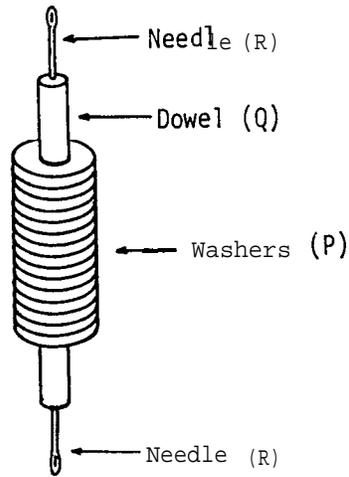
Slide the washers (P) onto the middle of the wooden dowel (Q). Add the washers until they make a stack 3.5 cm long on the middle of the dowel. Use epoxy resin to fix the washers in position. Drill a hole (0.1 cm diameter, 1 cm deep) into either end of the dowel. Cut two 2 cm lengths off the eye ends of the two needles (R), and insert these into the newly drilled holes (needle eyes projecting). Fix them firmly in position with the help of epoxy resin.
