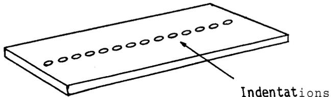
Make regular indentations down the middle of the top and bottom strips (A) of the framework, the indentations being 0.4 cm apart. These indentations can easily be made with a hammer and nail. The remaining two pieces of wood (B) will serve as sidepieces for the framework. Do not complete construction of the framework until the nails (C) are in place.
