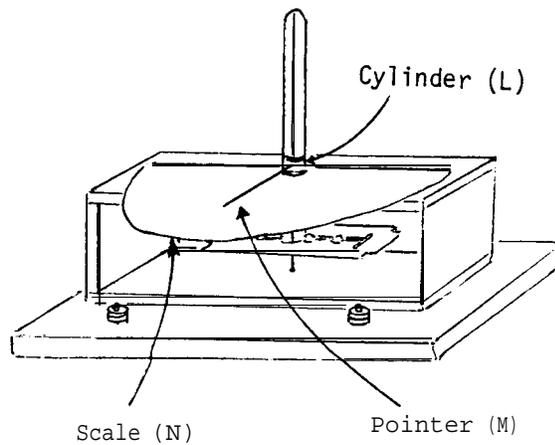
Cut a semicircular disc (diameter B cm) out of the cardboard sheet (N), and set it on top of the coil form to serve as a scale. Mark the position of the cardboard on top of the form, SO that the cardboard scale may be replaced in exactly the same position whenever it is removed.
