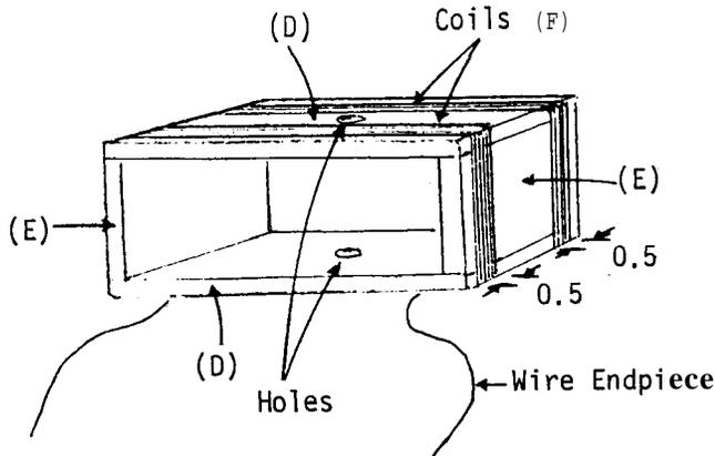
Make a wooden form using wood (D) for the top and base and wood (E) for the side pieces. Glue the pieces together.
