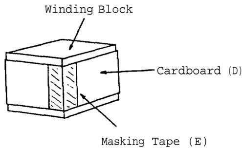
Wrap the cardboard loosely around the block fastening the two loose edges together with masking tape (E).
