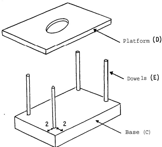
Make the base of the frame from wood (C) drilling holes (1 cm diameter) at the corners to take the dowels (E). Use wood (D) as a platform, drilling holes (1 cm diameter) at each corner to take the dowels. Attach the base and platform together by means of the four dowels, fixing the latter firmly in position with wood cement. Drill a hole (1.4 cm diameter) through the middle of the platform, making it just large enough to take the plunger.
