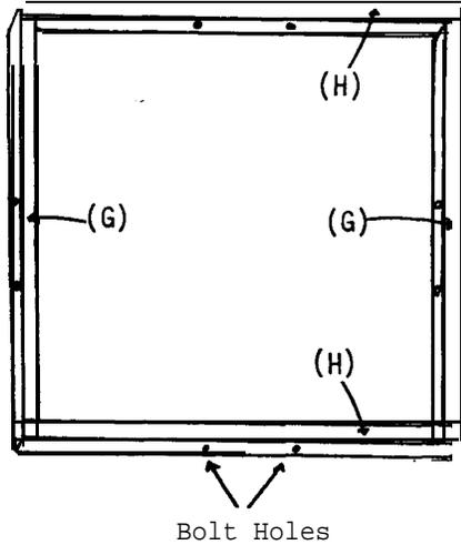
Use wood Strips (F) and (G) to make the frame of the plate support. Drill two bolt holes (0.3 cm diameter) in each side of the support, such that the holes in any one side are 4 cm apart, and are equidistant from the center of the side.
