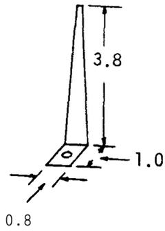
Cut two identical contacts out of the thin brass sheets (M) as shown. Attach these to the base of the apparatus with screws, so that they are in spring contact with opposite sides of the split halves.
