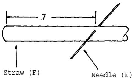
Insert the needle (E) through the top edge of soda straw (F) at a distance of 7 cm from one end. Balance the straw on the support.
