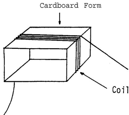
Wind 30 turns of magnet wire (E) around a cardboard form in order to make a coil of internal size 3.5 cm x 1.5 cm. Leave 10 cm of wire free at either end of the coil.
