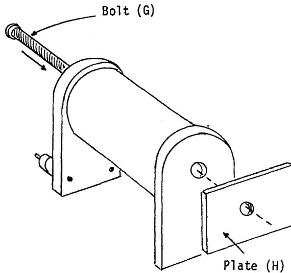
Drill a hole (0.4 cm diameter) through the center of the iron plate (H). Make a thread (0.4 cm diameter) in the hole, and attach the iron plate to the bolt (G) by means of the threaded hole.
