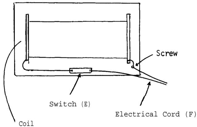
the double electrical cord (F) with two pin plug (G) attached, and connect one wire to the screw, and the other wire to the switch.
