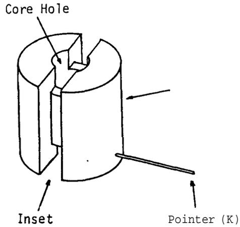
Make an inset (0.5 cm wide, 0.5 cm deep) around the wooden dowel (J) specifically to hold a coil. Drill a hole (0.8 cm diameter) along the axis to take the pivot and soft iron core.
