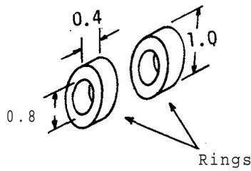
To make the AC commutator, cut two identical rings from the brass tubing (N).
