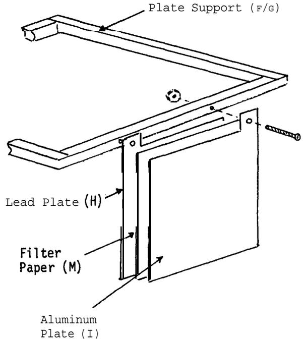
plate. Place the sheet of filter paper (M) between the two plates, thus insulating one from the other,
