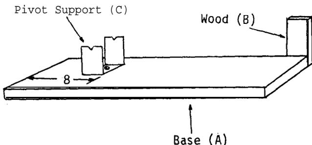
Fasten an upright piece of wood (B) to the rear of the base (A), and to one side. Make a pivot support from the sheet of aluminum (C). Drill a hole (diameter 0.2 cm) in the middle of the horizontal portion of the support, and attach it to the base with the screw (D).
