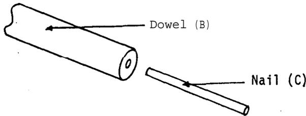
Bore holes into both ends of the wooden dowel (B) and insert long nails (C) into the holes to prevent the rod from floating in the ripple tank.
