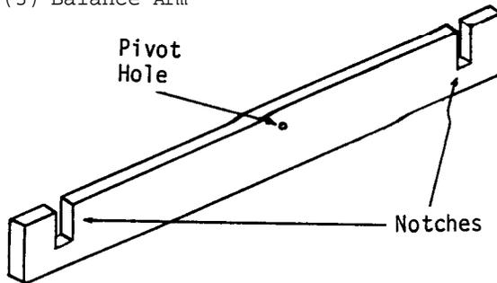
Make the balance arm out of softwood (G), cutting a notch (0.5 cm wide, 1.0 cm deep) at a distance of 1.5 cm from each end of the arm.
