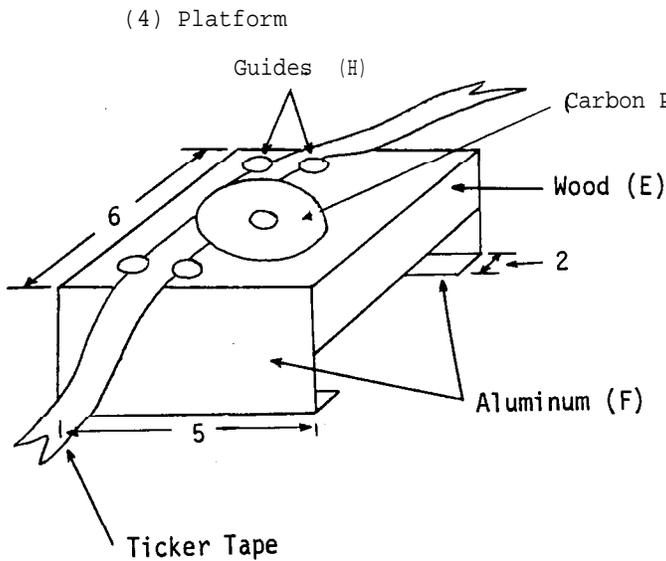
Attach the aluminum sidepieces (F) to wood (E) with nails to make a platform. Then with the platform in position on the base, bend the sidepieces at the bottom to hold the platform firmly in contact with the base. (A loosely fitting platform will result in a poor track being recorded on the ticker tape.)
