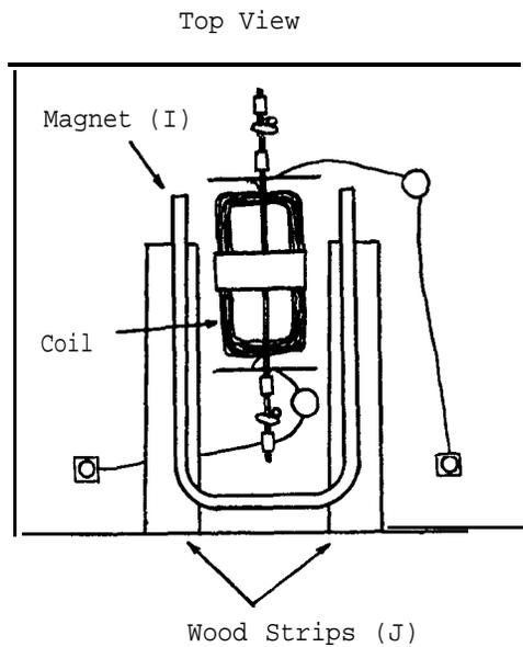
Procure a horseshoe magnet (I) with pole heads at least 4 cm apart, and place it as shown around the coil. Make two wooden strips (J) which, when placed under the magnet, will bring the pole heads up to the same height as the coil. The ends of the magnet should be located opposite the middle of the coil.
