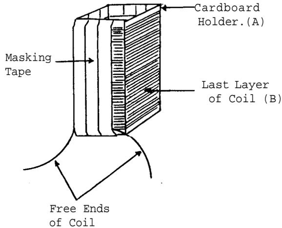
both ends. To do this a system of winding such as that described under IX/A2 should be adopted. (A variation is described in the notes below.) Wind the turns on to only the middle 6 cm or so of the cardboard holder. After winding each additional layer of turns, temporarily remove the cardboard holder (and turns) from the winding block, and cover the turns with masking tape. This not only holds the new layer of turns in position, but also insulates it from the next layer to be added.
