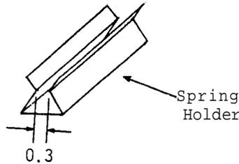
Make two spring holders from the two brass sheets (E) and slip these on the free ends of the multipurpose coils to determine where they should be attached to the upright. Having marked in the position, screw the
