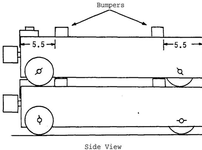
Use the two strips of wood (N) as bumpers. Nail them in position on top of the cart in such a way that they will hold a second cart (placed on top of the first) firmly in position.
