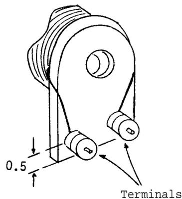
Drill a hole (0.6 cm diameter) along the axis of the dowel (A).
