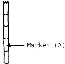
Mark off the end of wire (A) in half centimeter intervals (0-2 cm). The marker may then be used to determine the depth of the water at the four corners of the ripple tank, and makes the levelling of the tank simpler.
