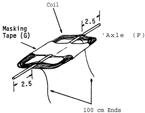
Thread the wire (F) through the middle of the coil to serve as the axle for the coil. Wrap masking tape (G) around the coil and axle to hold the coil firmly in position.
