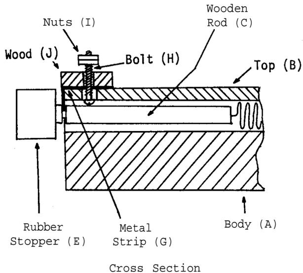
Bend the sheet of aluminum (G) into an "L" shape (8 cm wide, 2 cm tall, with a base of 1 cm). Attach the sheet to the front of the cart so that the base of the sheet just overlaps the slot for the spring device. **In this way** the spring may be compressed and held in position by means of the metal sheet and the notch in the rod.
