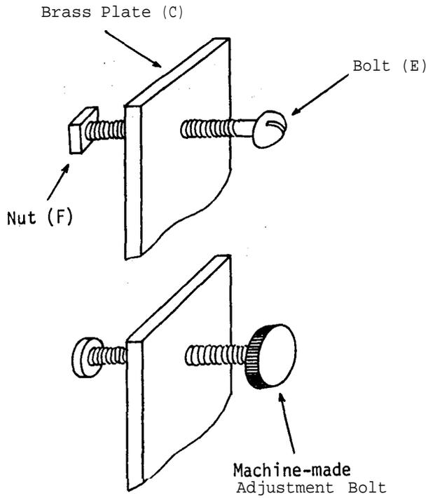
The latter bolt may have to be adjusted with the help of a coin, or some such device. A much more convenient adjustment bolt could be made by a technician, or anyone familiar with a metal lathe, cutting the head and bolt from a single piece of brass. The base in either case would be made from a separate nut (F), firmly attached to the bolt by damaging the threads at the end.
