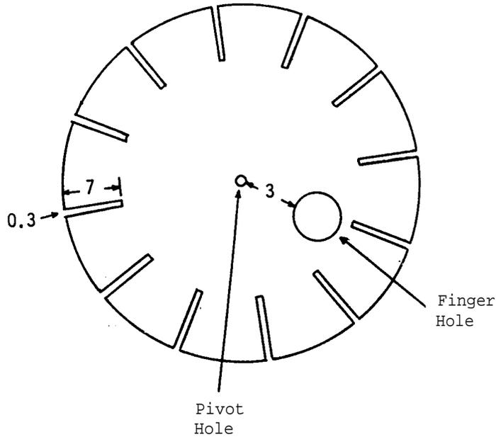
Cut the stroboscope wheel from the piece of hardboard (A). Make 12 equally spaced slits in the perimeter of the wheel. Drill a finger hole (2 cm diameter) at a distance of 3 cm from the center of the wheel, and a pivot hole (0.5 cm diameter) at the center of the wheel.
