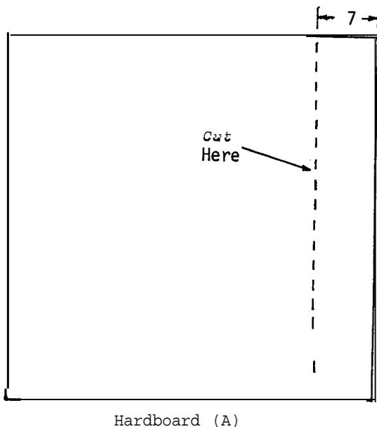
Cut a 7 cm strip from one side of the plywood (A), and shape the newly cut edges back at an angle of 45° as illustrated. Reattach the 7 cm strip to the platform with very small hinges (B) avoiding the creation of a gap between the strip and main platform. Shape the free edge of the 7 cm strip to an angle of 45°. This shaping insures good contact between the strip and the table.
