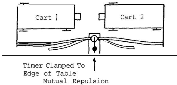
The purpose of the bracket is to insure that ticker tape attached to the cart is in line with the guides of the timer during any experiment, thus reducing friction. Two typical examples are illustrated when carts are mutually repulsed from one another, and when a single cart runs down an inclined plane.
