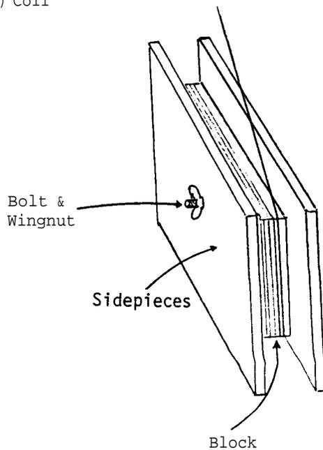
To make the coil a simple winding device is desirable. This may be made from a block of wood (5 cm x 5 cm x 1 cm) and two cardboard sides (8 cm x 8 cm x 0.5 cm). Drill a hole through the middle of the block and sides and hold the parts together with a bolt and wing nut.
