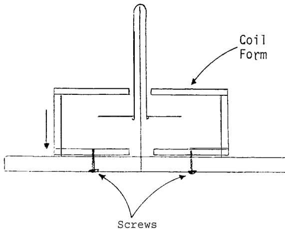
Lower the coil form and tube together onto the needle projecting vertically from the base. Take two screws (K) and firmly attach the base and coil form together.
