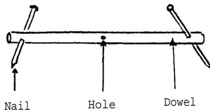
case 1.4 cm diameter, 30 cm long) with a hole (0.6 cm diameter) drilled at either end to take a nail about 10 cm long.
