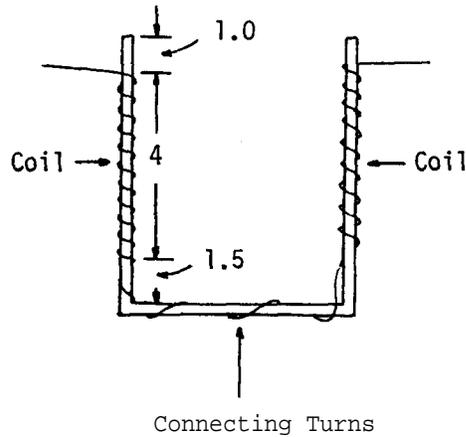
and attach the free end of the wire to one of the front terminals as indicated.
