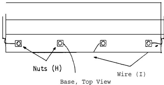
Use copper wire (I) to attach the end terminals to the end-pieces, fastening the bare ends of the wire beneath the terminal locking nuts and brass endpieces. Similarly attach a length of copper wire (I) (15 cm long) to each of the middle terminals.
