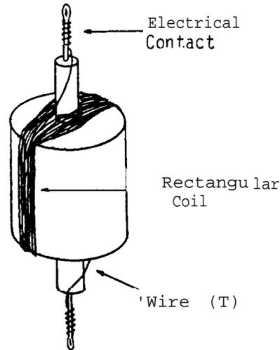
Take the magnet wire (T) and wind it around the dowel (S) to make a rectangular coil contained within the groove which was cut for this purpose. Bare the ends of the wire, and wrap them around the stem of the top and bottom needles (R) respectively, insuring good electrical contact between magnet wire and needle.
