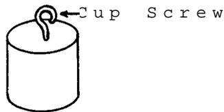
The lead cylinders may then be filed down until each is the desired mass. The number of masses required, and the
