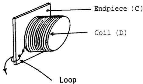
Drill a small hole in each endpiece and loop the wire ends through these holes to prevent unwinding of the coil.
