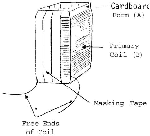
To make the primary coil, wind 720 turns (approximately 250 g) of magnet wire (B), onto the cardboard form. Each layer of turns will be 10 cm long. Place masking tape between each layer. The actual method of winding is described under VII/Al.
