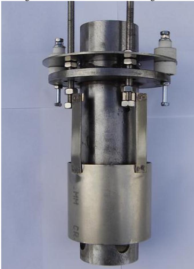
2. A NiCr heating element scavenged from the same heater wound around fibreglass matting and providing 300W of power. The fibreglass was held in a wound state around the outside of the cell by two stainless steel hose clips. Each of the hoseclips also acted as a terminal for
