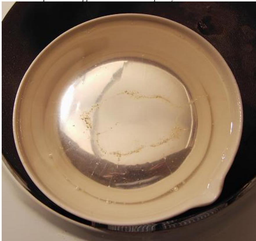
Initially the cell was run for 150 minutes at an average current of 47A, resulting in 24.6 gms of crude Na. Assuming 1 gram of the weight is bath crud that gives a yield of 23.6 grams. Now 96000 Coulombs at 100% current efficiency give 23 grams of Na. In our case
