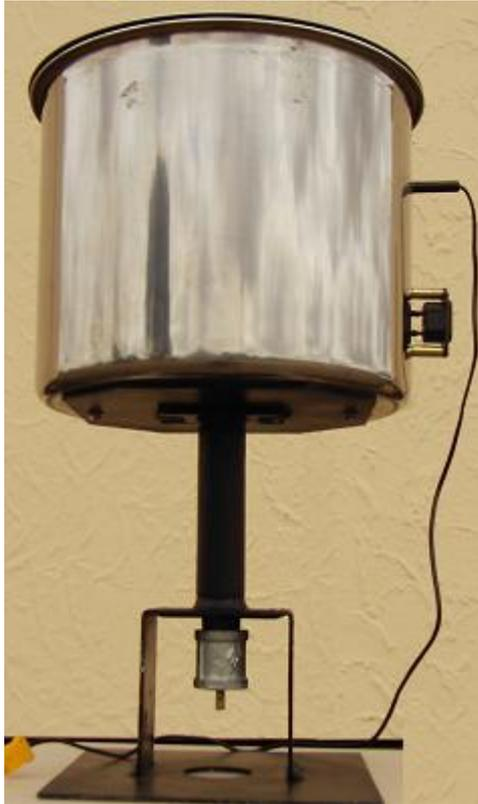
7. The cathode was 5cm long 15mm diameter wound copper tubing. Fixed at the bottom (cool end) to a threaded nut and sealed with exhaust cement. See figure 9.
