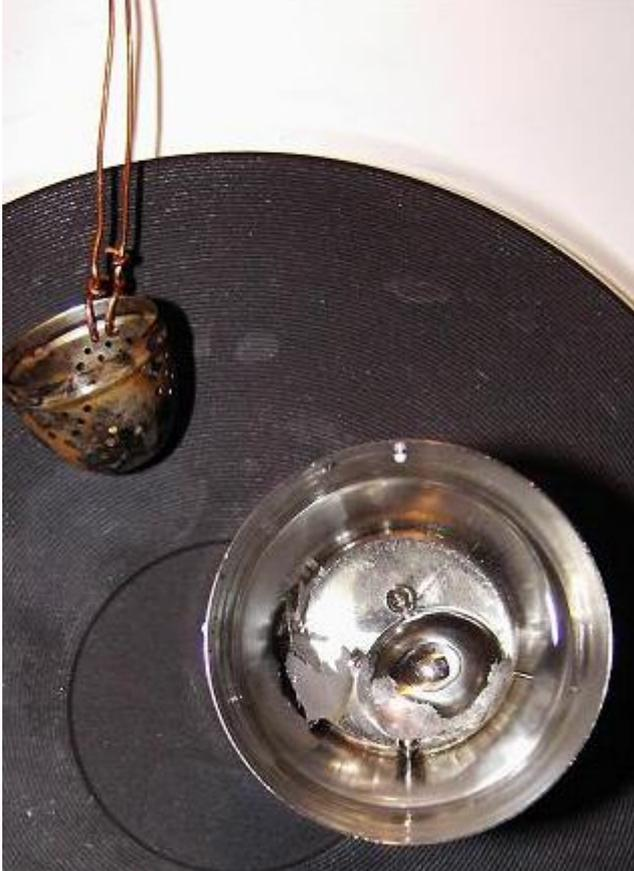
10. The bath current was 47 - 50A. Experiment time was about an hour to produce the sodium shown.
