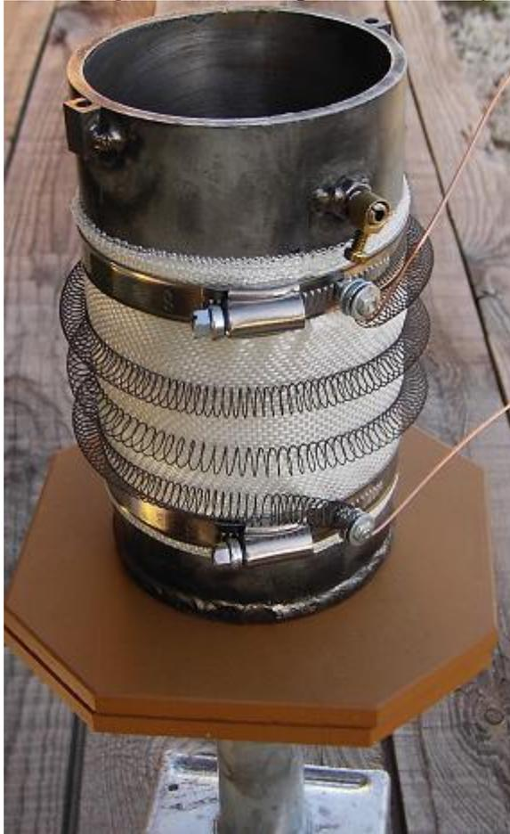
3. An outer radiative-heat container of SS (an indian coffee jar from woolworths) of 15cm diameter and 15 cm long encased the cell with wound NiCr. See figures 5 and 6.
