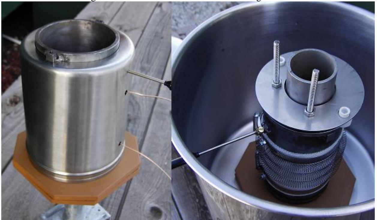
4. Holes drilled in the radiative container with terminal posts attached to bolts drilled in the hose clamps allowed the passage of heating current at 240V. Note its independent of electrolysis current, and is only needed at startup. A hole also passed a thermocouple probe
