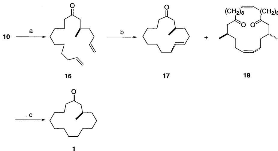
**Scheme 4.** Reagents and conditions: (a) Jones reagent, CH<sub>3</sub>COCH<sub>3</sub>, 5 min; (b) 5 mol% of **2**, CH<sub>2</sub>Cl<sub>2</sub>, 21 h, 45°C; (c) H<sub>2</sub>, 10% Pd-C, MeOH, 3 h.
