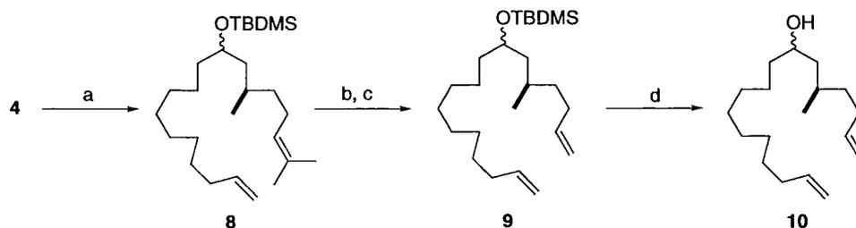
**Scheme 2.** Reagents and conditions: (a) TBDMSCl, imidazole, DMF, 21 h; (b) O<sub>3</sub>, CH<sub>2</sub>Cl<sub>2</sub>, -78°C, Me<sub>2</sub>S, -78°C then rt, 12 h; (c) Ph<sub>3</sub>PMeBr, *n*-BuLi, THF, -78° then rt, 4 h; (d) TBAF, THF, 24 h.
